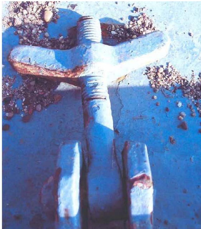
Figure 25: Example of unserviceable hatch dogs found on the ELIZABETH M. Heavy paint would make it impossible to properly secure a hatch.
