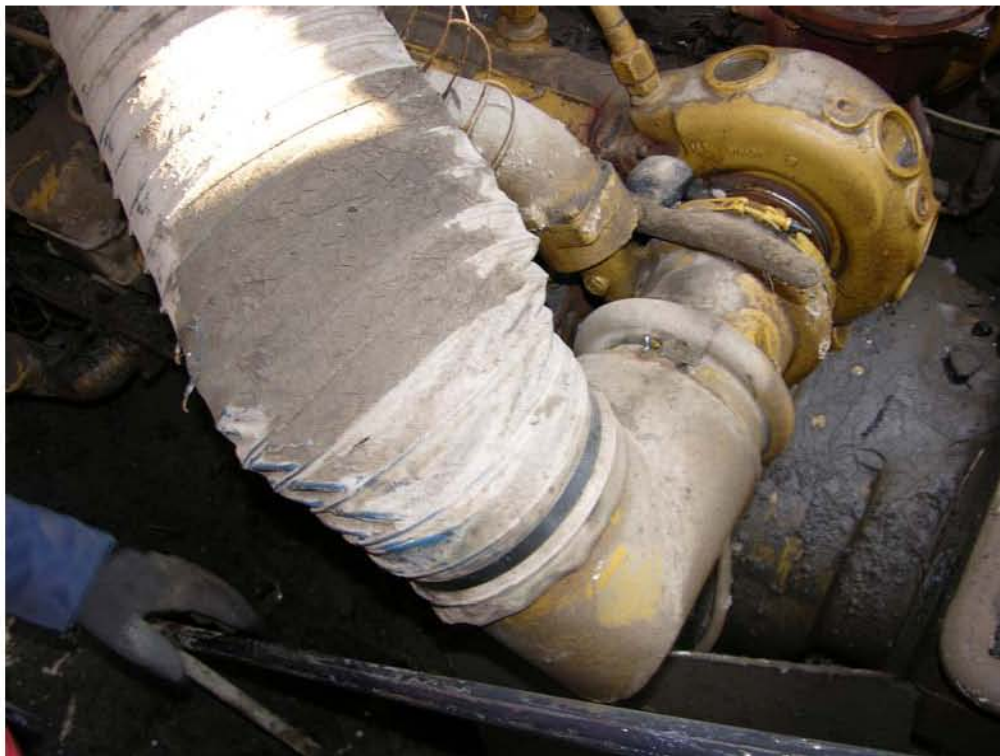
Collapsed PVC hoses at a MDE turbocharger inlet.
