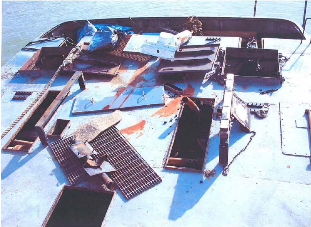
Figure 25: Example of unserviceable hatch dogs found on the ELIZABETH M. Heavy paint would make it impossible to properly secure a hatch.
