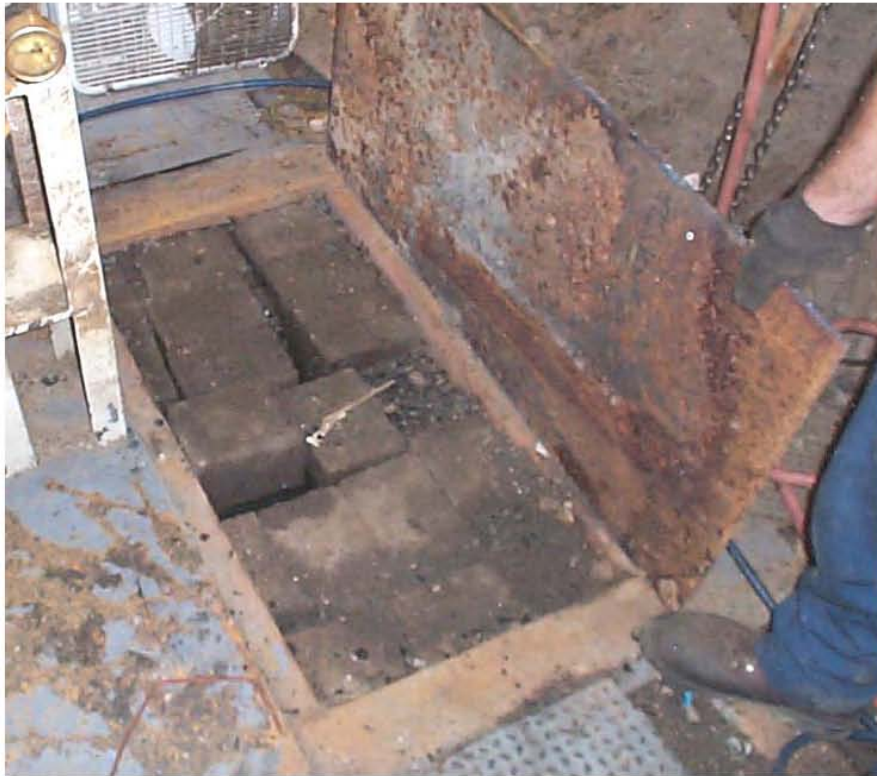
Figure 4: Post-casualty photographs of ballast installed in the engineroom on the ELIZABETH M in April 1997.
