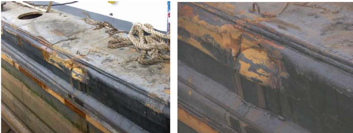
Figure 5: Post-casualty photographs of ELIZABETH M rub rail damage sustained on 31DEC04.
