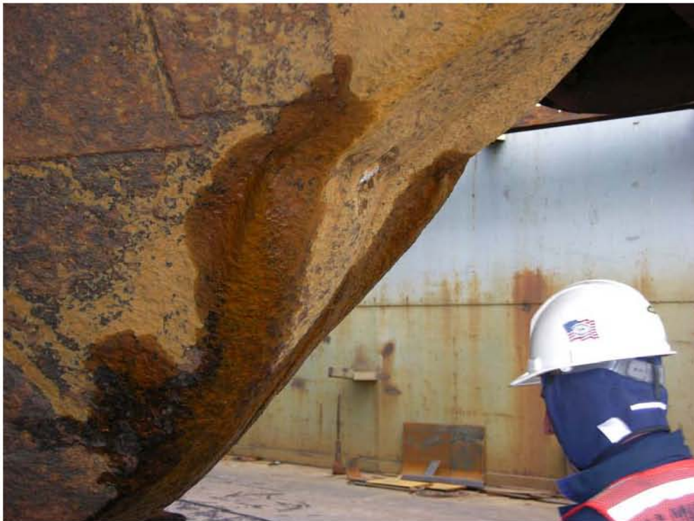
Figure 23: Post-casualty photograph of pinholes and fractures in The ELIZABETH M forepeak.
