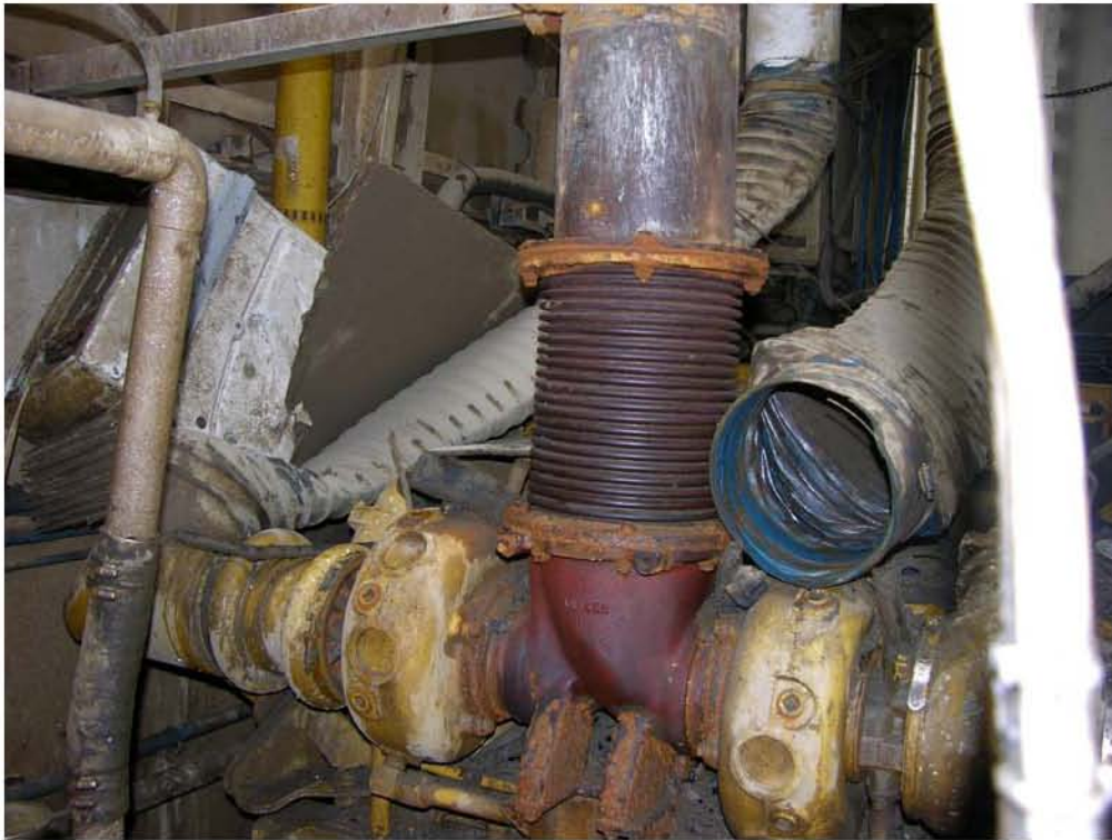
Collapsed PVC hoses at MDE turbochargers inlets.
