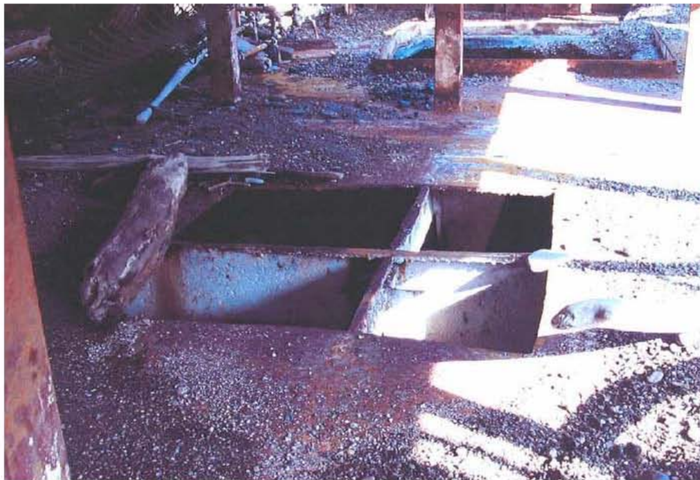
Figure 26: Post-casualty photographs of the two 25" x 25" cutouts in ELIZABETH M's main deck.
