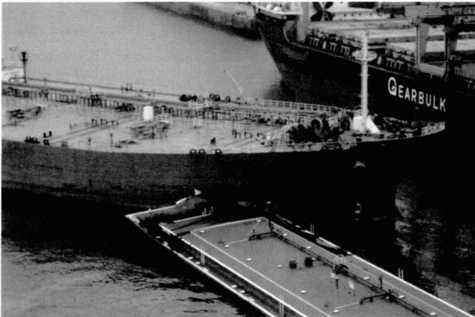
Figure 2: Closer view of post collision positions of EAGLE OTOME, KIRBY 30406 and GULL ARROW. Also visible is the damage to the GULL ARROW on the hull at the juncture of the deck with the house (white superstructure).
