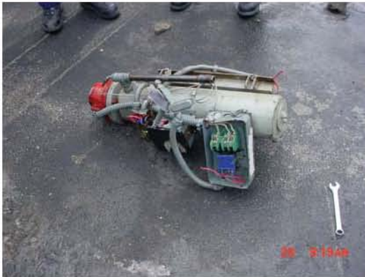
Figure 5-8: Electric fuel heating unit
