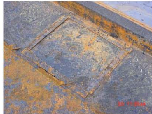
Figure 5-35: Cargo tank top repairs
