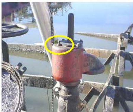
Figure 5-17: Cargo tank #1 P/V valve
