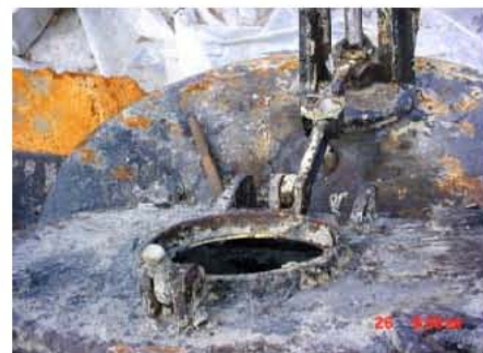
Figure 5-4: Ullage opening/Sounding port
