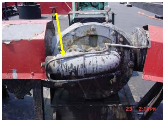
Figure 5-26: EMC 427 Cargo pump with heat trace tubing
