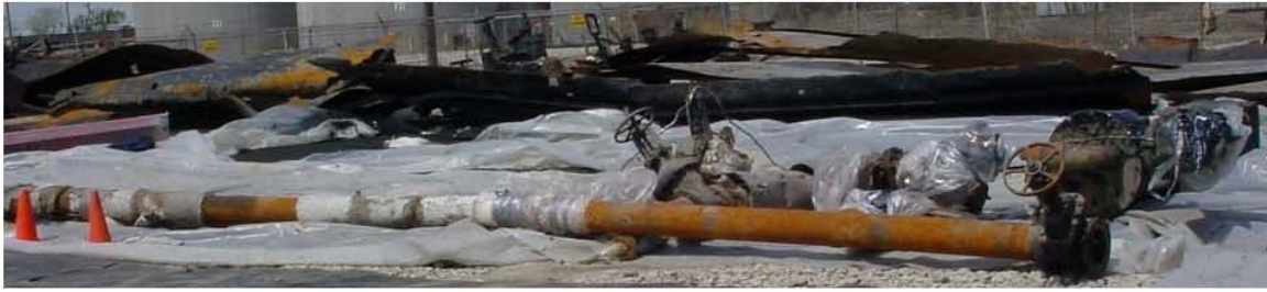
Figure 5-25: Reconstructed transfer header, loading and discharge piping including cargo pump
