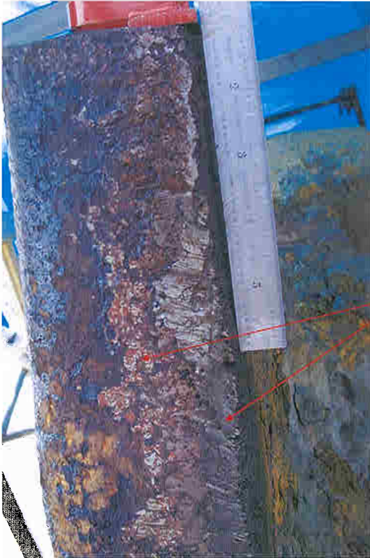
Anchor Blade – showing the metal scrapes and red paint rubs.
