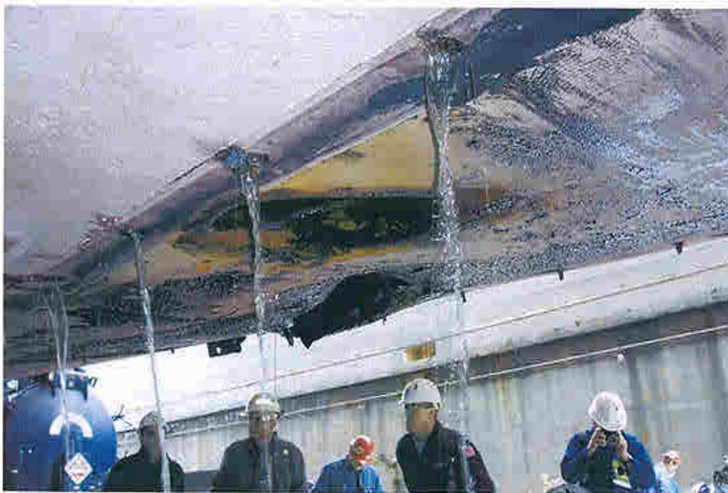
Main External Damage of the ATHOS I hull
