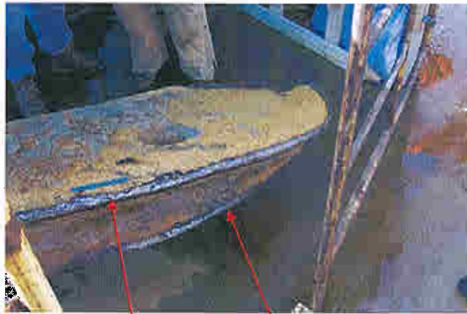
Anchor Fluke – notice the metal scrapes along the sides
