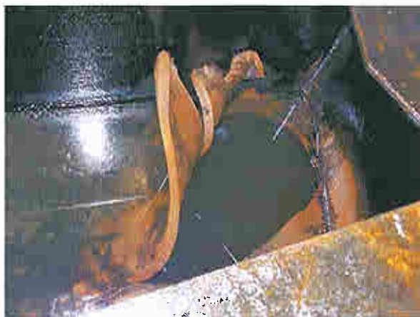
Puncture Damage located in the #7 Center Cargo Tank. ** Viewed from inside the tank **
