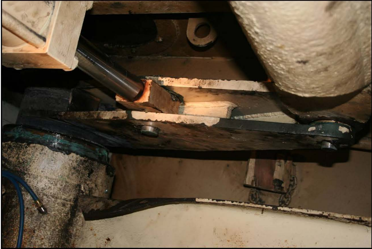
Figure 30: Steel Tiller Assembly showing hydraulic steering system connection and cross connect (from M/V DEFENDER)
