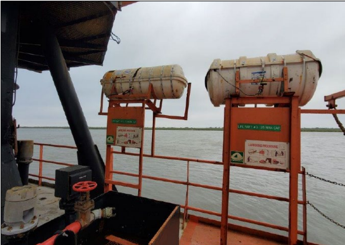
Figure 47: Liferafts stowed on SEACOR POWER (Exhibit 202)
