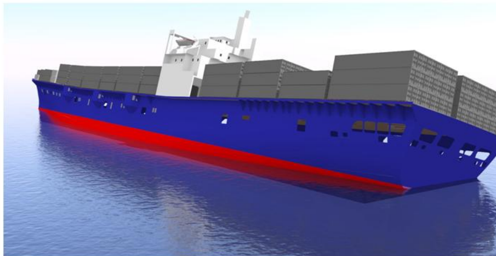
Figure 9. EL FARO computer rendering with 15 degree starboard list and trimmed down by the stern 5.8 feet, due to flooding of Hold 3 estimated at 20% and wind heel. Illustration produced by the USCG Marine Safety Center.
