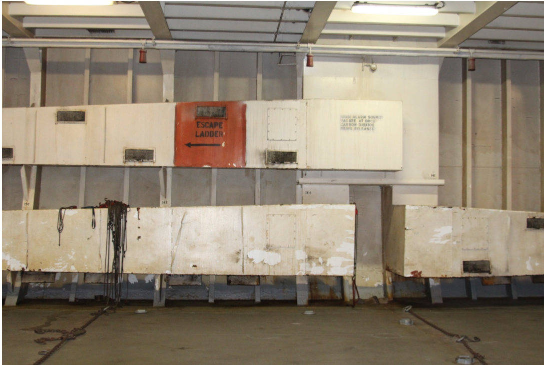
Figure 6-13: Ventilation supply plenums inside Hold 3, frames 141-144 port, 4 th deck (tanktop, innerbottom). Photo of sister vessel EL YUNQUE. USCG photo.
