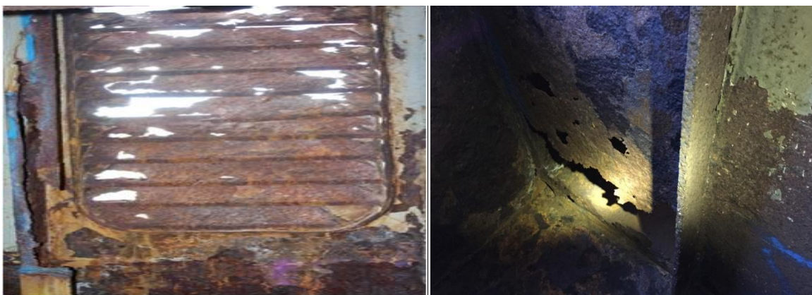
Figure 28. Photographs taken by Coast Guard Traveling Inspectors during an October 2016 visit to EL YUNQUE in Tacoma, WA showing examples of corrosion within the vessel’s exhaust ventilation trunks. (U.S. Coast Guard photographs)
