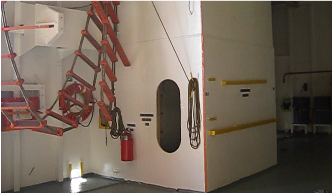
Figure 6-11: Hold 3 aft ventilation exhaust trunk with racking bulkhead, frames 159-162 starboard, 2 nd deck. Screen capture from video taken September 2008 provided by Tote, Inc.
