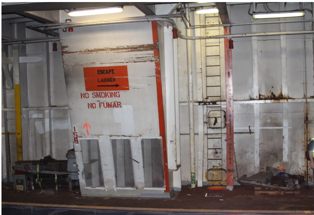
Figure 6-14: Ventilation exhaust intake plenum inside Hold 3, frames 159-162 starboard, 3 rd deck. Hold 3 starboard scuttle personnel access ladder and remote operator rod for the emergency fire pump suction valve (sea-chest isolation) are shown on the right. Photo of sister vessel EL YUNQUE. USCG photo.
