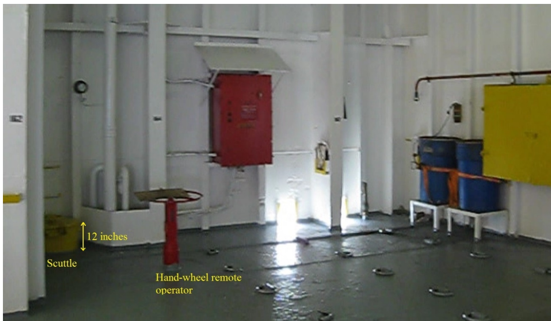
Figure 6-6: Hold 3 (also called Hold D) starboard personnel access scuttle on the 2 nd deck at frame 163. Note that the scuttle opening is 12 inches above the deck. The hand-wheel remote operator for the emergency fire pump sea-chest isolation valve is also shown. Screen capture from video taken aboard EL FARO September 2008 provided by Tote Inc.
