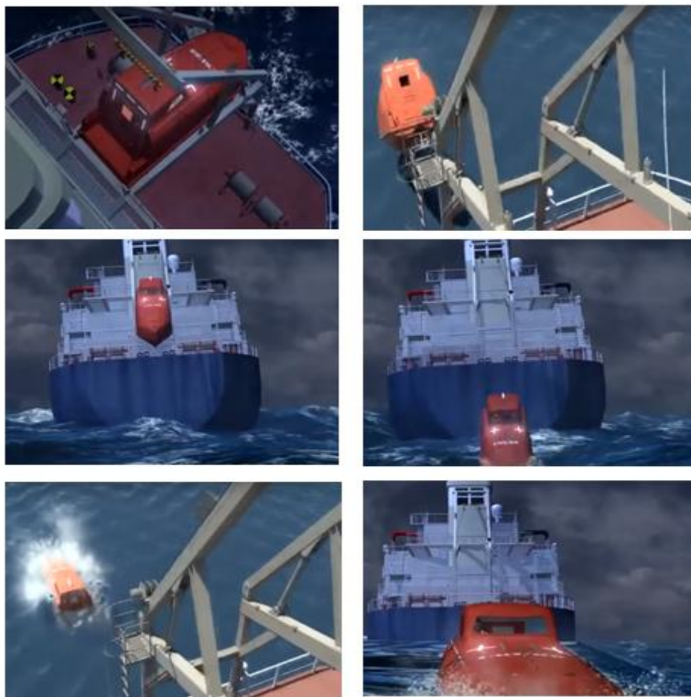
Figure 48. The launching sequence for a gravity launch, free-fall lifeboat arrangement. Upper left, crew enters boat and straps in. Boat is released and enters the water where the kinetic energy propels the boat clear of the ship. The engine is running when the boat enters the water. (Source: Karishma Marine Solutions Pvt Ltd (KARCO), India)
