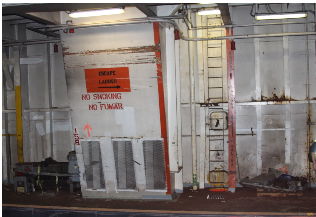
Figure 6-14: Ventilation exhaust intake plenum inside Hold 3, frames 159-162 starboard, 3 rd deck. Hold 3 starboard scuttle personnel access ladder and remote operator rod for the emergency fire pump suction valve (sea-chest isolation) are shown on the right. Photo of sister vessel EL YUNQUE. USCG photo.
