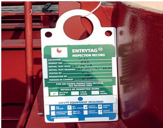
Figure 2: Entry tag displayed on entrance to enclosed space. This summarises that the space has been passed for entry by a competent/responsible person.
