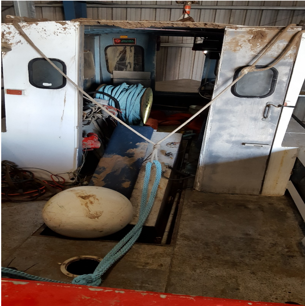
Figure 4. CAJUN SPECIAL's towline configuration as it was on the day the incident occurred. Photo taken after salvage of the vessel. Tow bridle is attached to handrails on top of wheelhouse. The blue towline goes aft over the transom (stern) of the vessel and should be under a fairlead (line) that is attached to cleats on the port and starboard aft gunwales to bring the towline low. The fairlead was missing. (February 26, 2018/USCG)
