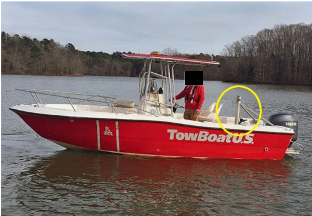
Figure 3. Example of standard tow configuration for assistance towing. The yellow circle shows the specific point of hook-up for the towing line. (December 12, 2018/Google)
