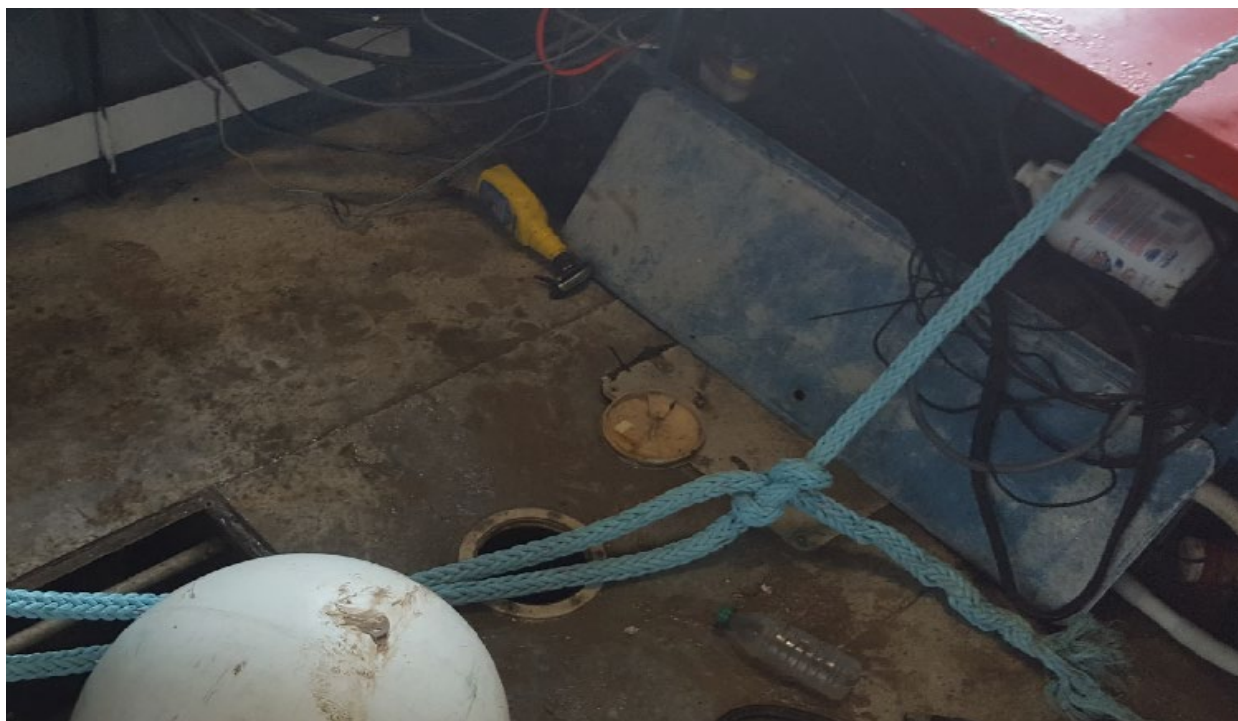
Figure 2. Towing bridle coming from top of wheelhouse, with severed line, coming over the stern of the vessel, tied to it. Photo taken after vessel was salvaged. (February 27, 2018/USCG)
