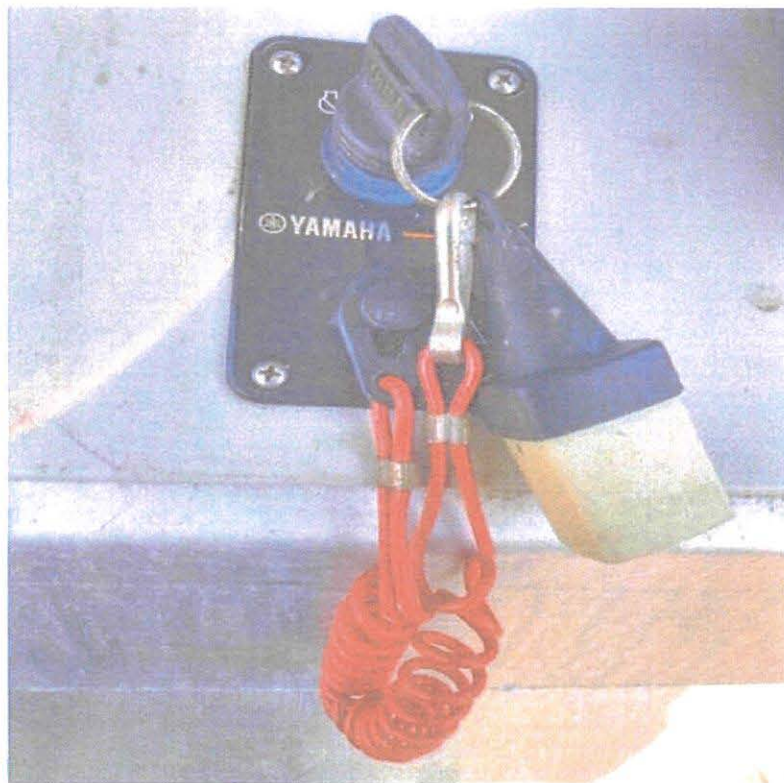
Figure 3. SEA MULE engine safety ignition cutoff switch taken on November 19, 2022 by USCG
