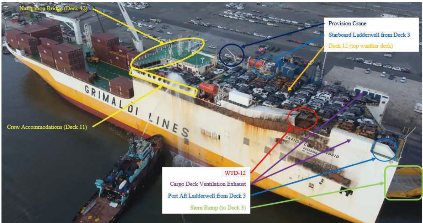
Figure 8. Port aspect of GRANDE COSTA D'AVORIO post-fire indicating significant areas of the vessel. Developed by Coast Guard Investigators.
