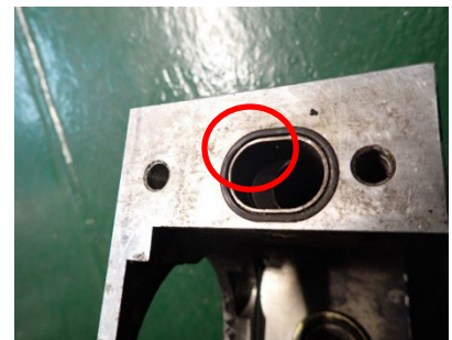
Pinched Seal on the Oil Flow Meter Block
