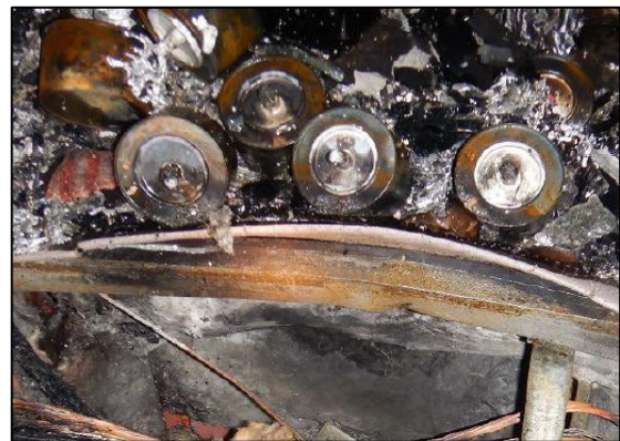
Figure 2: Post fire images of Sterno® cans stored in server station of the vessel.
