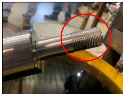
Photographs taken of disassembled ram showing rod stud threads and retaining nut.
