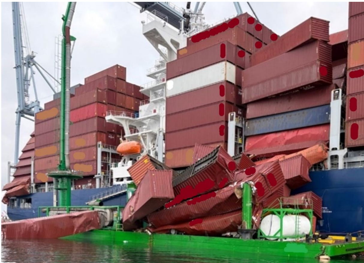
Fallen containers on an emissions control barge that was moored alongside a container vessel during cargo operations.
