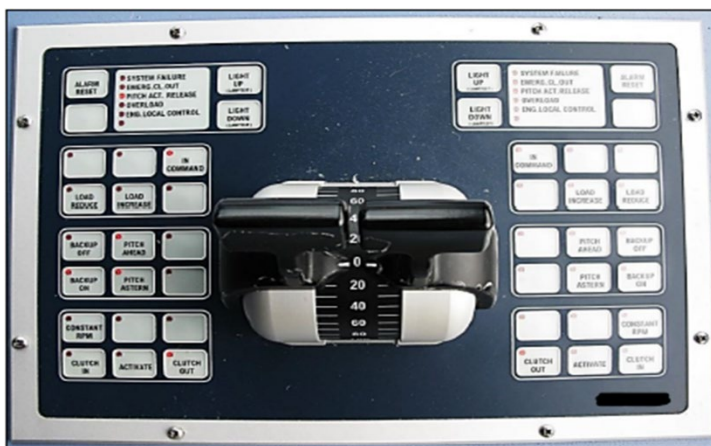
Figure 1 – Vessel bridge maneuvering control panel.
