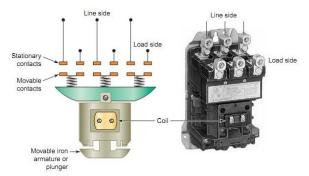
Figure 1: Typical magnetic motor contactor (Image credit: www.industrial-electronics.com)
