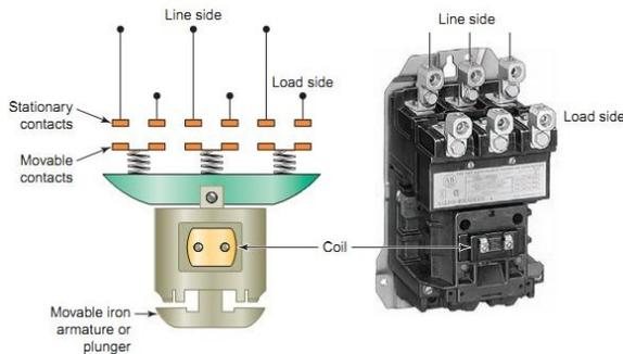
*Figure 1: Typical magnetic motor contactor
