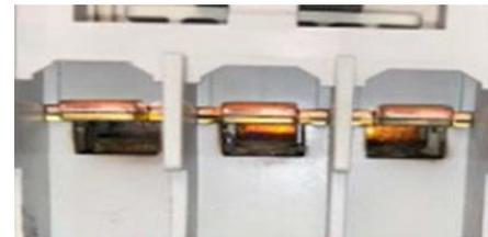
*Figure 2: Welded contactors
