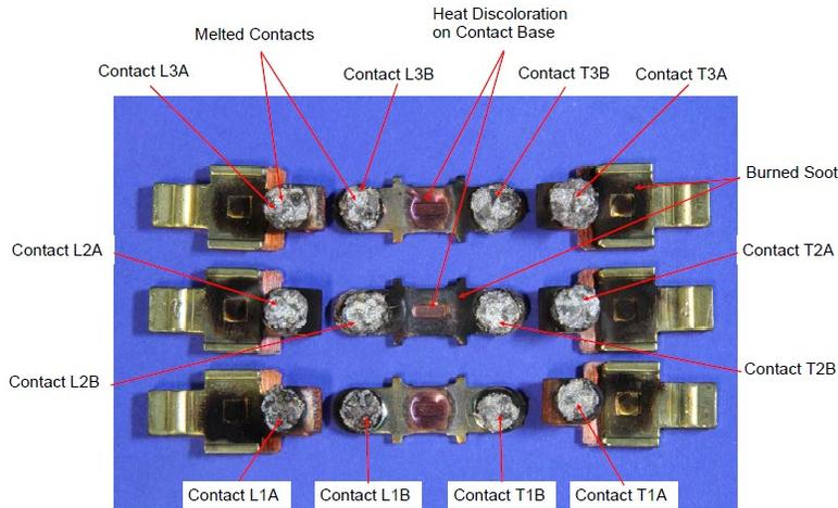
Figure 3: Disassembled contactor during forensic analysis
