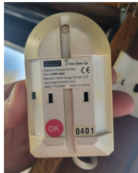
Figure 2: Passive Infrared Sensor installed on the towing vessel.
