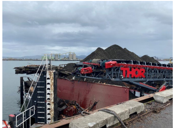
Figure 1: Damage to fully loaded barge and towing vessel, after alliding with bulk liquid transfer terminal pier.
