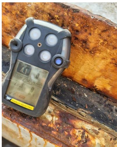
Figure 2: Portable gas meter with levels of H<sub>2</sub>S detected upon removal of bilge covers.
