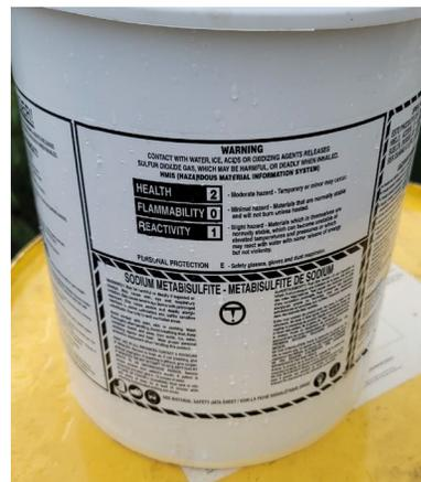
Figure 3: Warning label on a bucket of Sodium-Metabisulfite.
