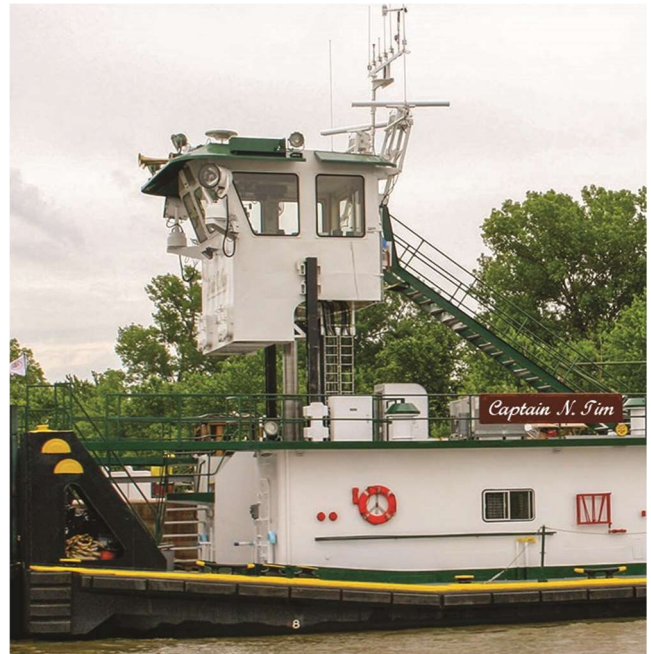
Towing vessel with a retractable pilothouse. Photograph courtesy of WaterwaysJournal.net Note: This is not the vessel associated with the casualty that led to the development of this alert.
