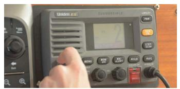
4. Re-adjust the VHF radio's squelch control until the audio noise is quiet, only slightly above the noise threshold.
