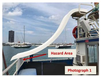
The slide in Photograph 1 above is of the open flume design. Closed flume slides (e.g., tubular designs) help to prevent users from contacting components external to the slide.
