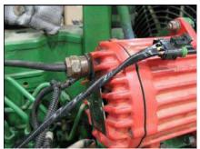
In some installations, cables between the alternator and battery were cut and a connector put in place to allow easier servicing. This alteration is not appropriate for hazardous locations. The cable seal on this alternator may not be the one approved for the alternator and may have to be examined.
