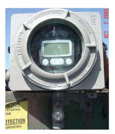
Typical acceptable electronic display – This particular one was approved by the Marine Safety Center (John Deere Part No. RE531478)
