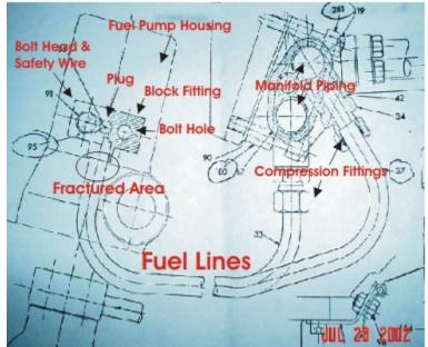
bolts are drilled to receive safety wiring which when properly used prevents loosening. Also located on each block fitting directly between the two bolt holes is a viewing plug that is removed whenever necessary to time the fuel pump to the engine.
