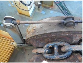
As an added safety device, a wire sling had been used to secure the anchor. The wire sling was threaded through a chain link and secured to the vessel with a pelican hook. When the sling broke and the brake failed, the anchor's weight and ship's movement then caused it to drop before the riding pawl could properly engaged.
