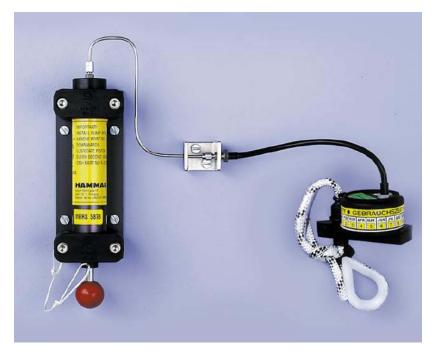
MRRS pump units are clearly marked black letters on yellow а background on the cylinder housing, "Lubricate piston every second year." The pumps that failed had not been lubricated as required. malfunctioning MRRS pumps were replaced in kind with new units; USCG inspection showed that the units new operated properly. Owners, operators, port engineers, inspectors and others involved in vessel safety should ensure that all appropriate steps are taken to properly maintain survival equipment.
