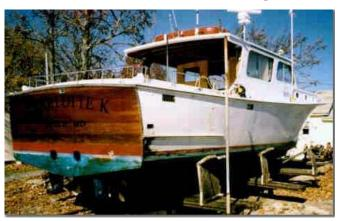
Upon return from a routine day fishing trip in November 1997, the operator of an inspected wood small passenger vessel reported that his vessel was taking on water at the dock after discharging passengers. Preliminary investigation indicated that the starboard chine log and outside starter plank of his 41 ft crossplanked Chesapeake deadrise hull were fractured.
