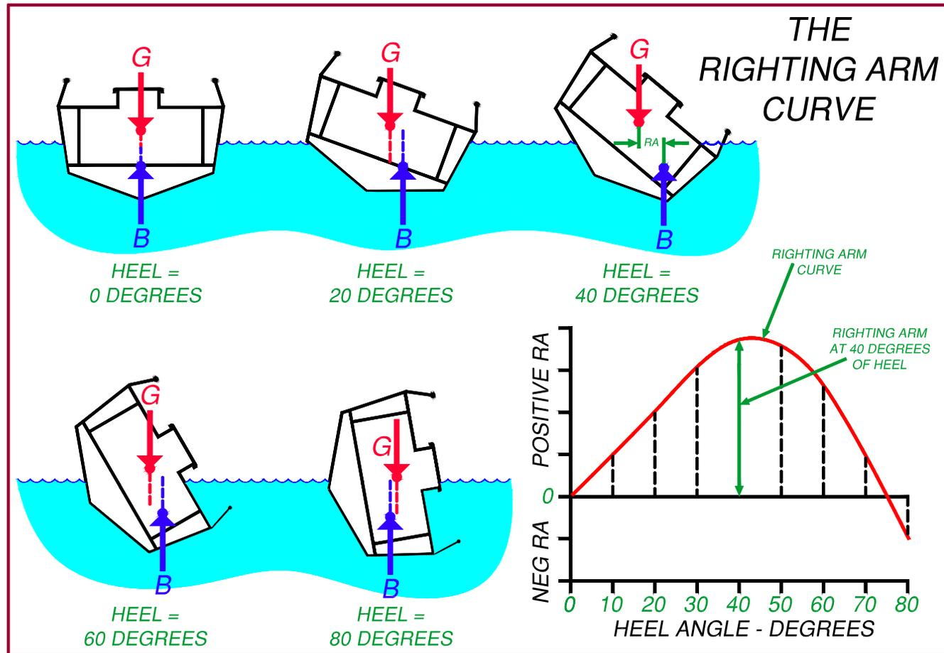
The righting arm curve has the heel angle in degrees plotted on the horizontal axis and the righting arms plotted on the vertical axis.
