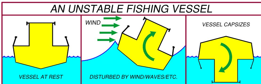
A fishing vessel is called **unstable** when it does not have enough positive stability to counter the external forces generated by current weather and fishing conditions and capsizes.
