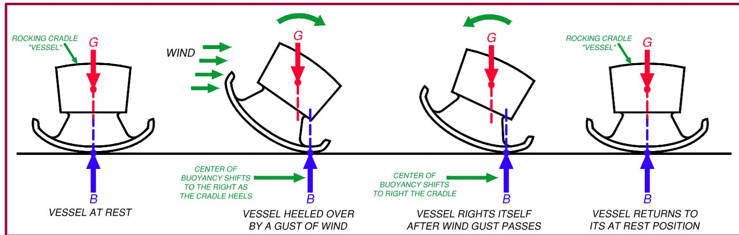
As with a fishing vessel, the cradle’s (vessel’s) center of gravity “G” is above its rocker, the center buoyancy “B”. The slightest disturbance (wind, waves, or the movement of weight on the deck) causes the cradle (vessel) to roll (heel) to one side.
