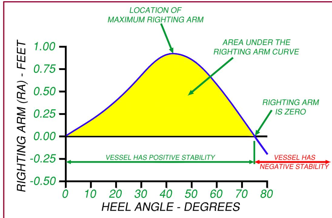
3) The maximum righting arm is an indication of the fishing vessel's ability to counter capsizing moments at high heel angles. In general, the larger the maximum righting arm and the higher the heel angle at which the larger the storms or capsizing moments the fishing vessel can handle.
