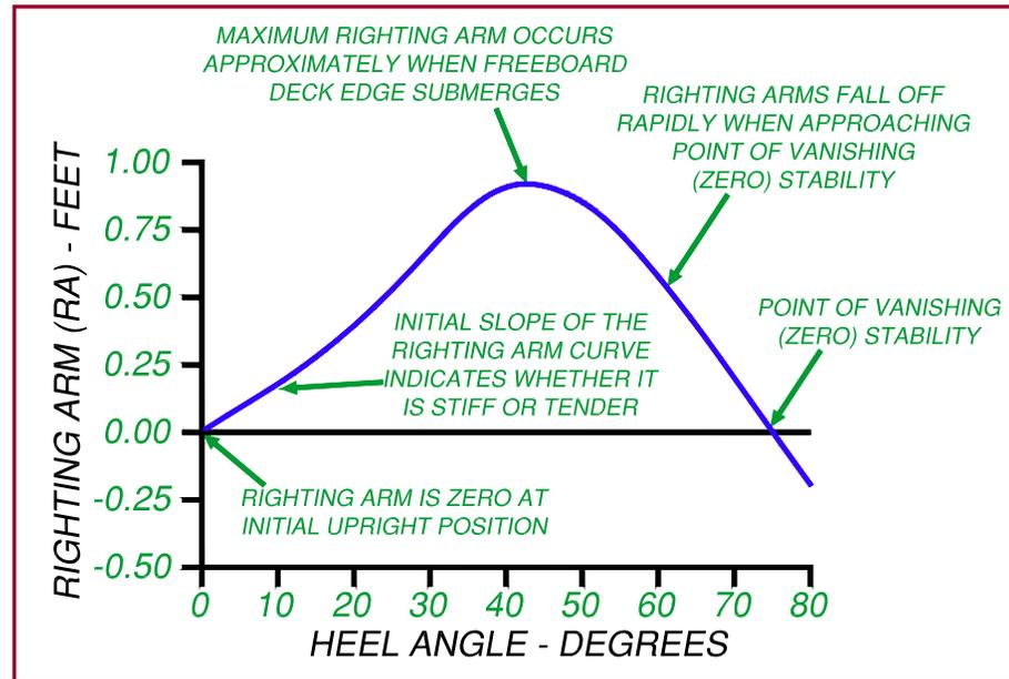
The shape of the righting curve at low angles of heel indicates how the vessel responds when subjected to low to moderate wind and waves.
