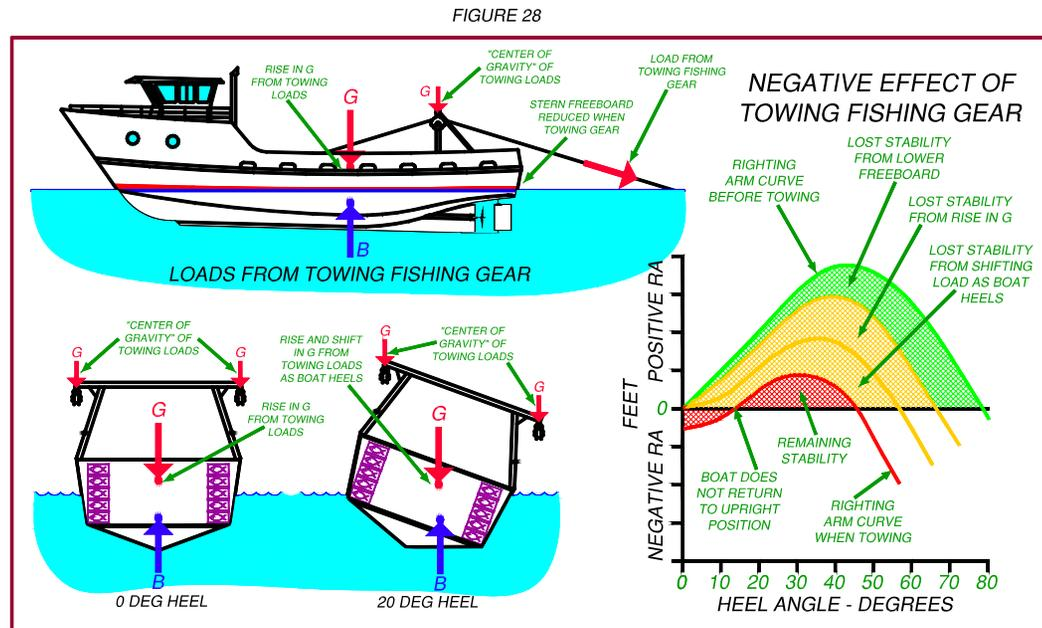
Recommendations: Tow directly off the vessel's stern using the lowest towing point possible.
