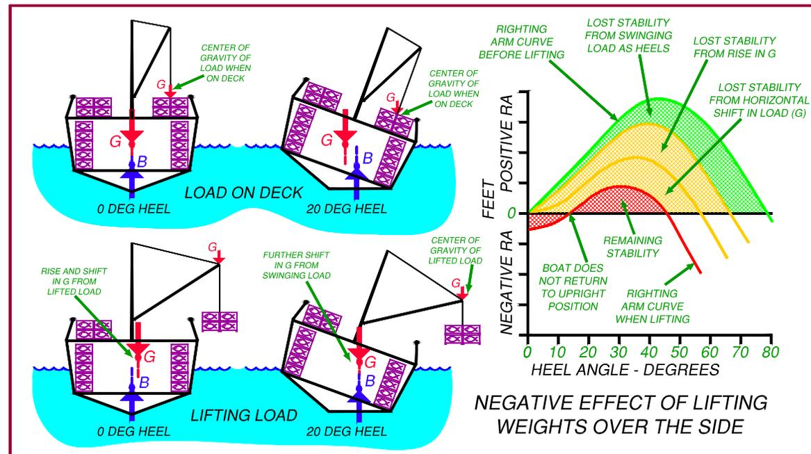
**Recommendations:** Never lift more weight than recommended in the vessel's stability guidance. Minimize the time when lifting fishing gear over the side of the vessel and if possible secure the load to prevent excessive swinging. If seas are moderate to large, suspend all lifting operations and secure the all fishing gear and catch to prevent its shifting.
