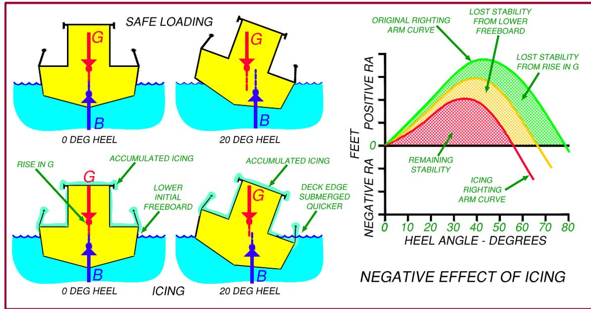
Recommendations: When icing conditions are encountered immediately take appropriate corrective action in any of the following procedures:
