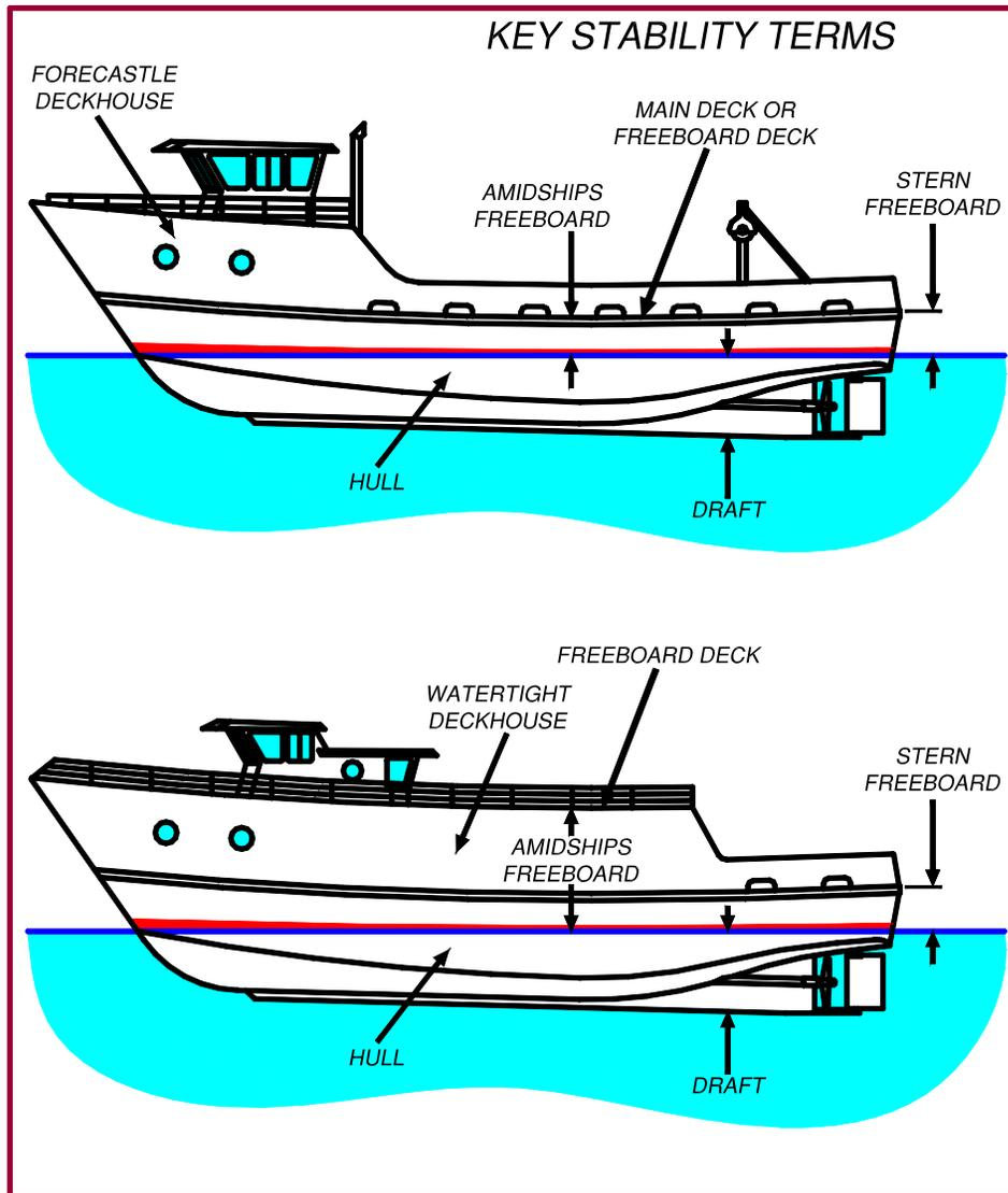
**Hull** - The enclosed portions of the vessel below the highest watertight deck that runs continuously from the bow to the stern. In most fishing vessels, the main deck is the highest watertight deck.
