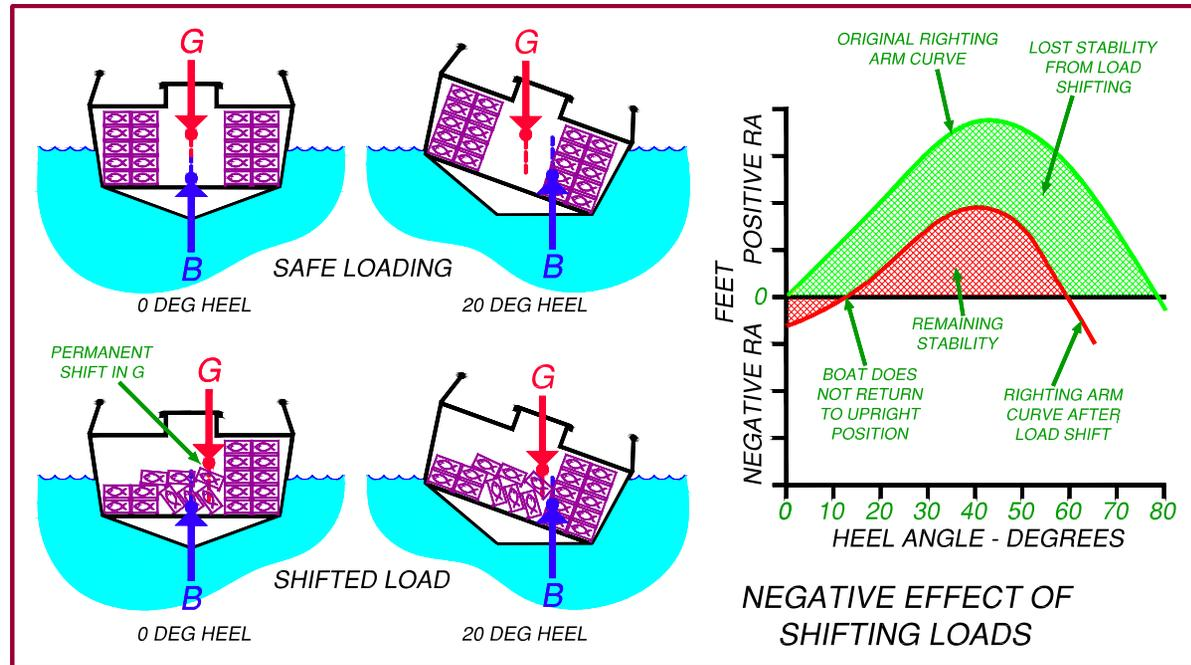
Recommendations: Secure all catch to prevent shifting. Also secure all fishing gear and other heavy items when not in use to prevent their unintended movement.
