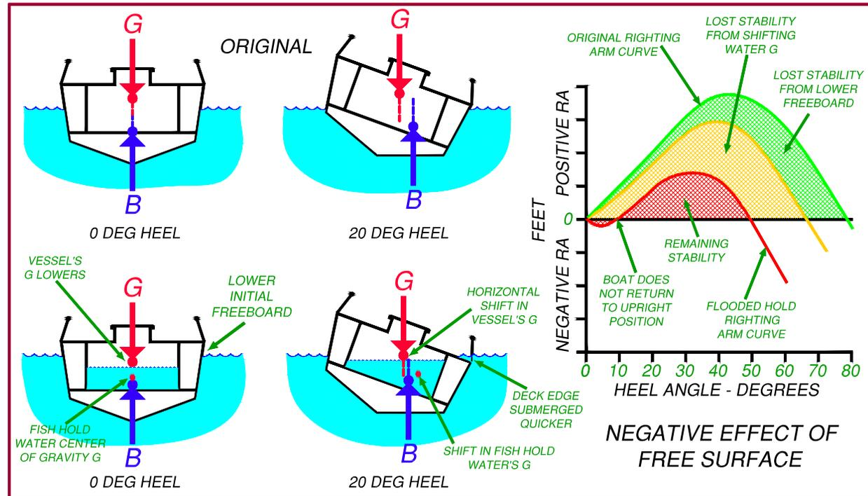
The diagram shows how the overall stability is reduced because the water in the hold has sloshed to the low (outboard) side. This shift causes the vessel's center of gravity "G" to shift farther outboard leading to a reduction in the vessel's righting arm curve. This reduction is significantly larger for very wide tanks or compartments that span the full beam of the vessel than for narrow wing tanks.
