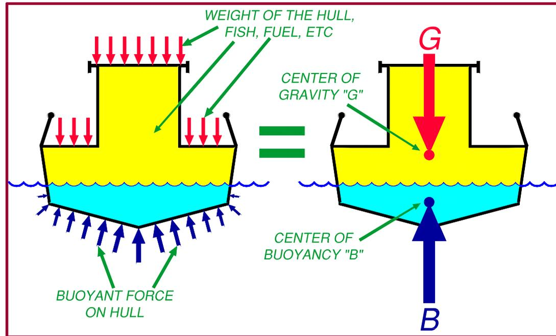
**Buoyancy** is the force acting to push the vessel up in the water; making the vessel float. In stability analysis, the total buoyancy forces, which are distributed over the part of the hull below the water, are mathematically combined into a single point called the Center of Buoyancy. This point is labeled "B" on stability model diagrams.
