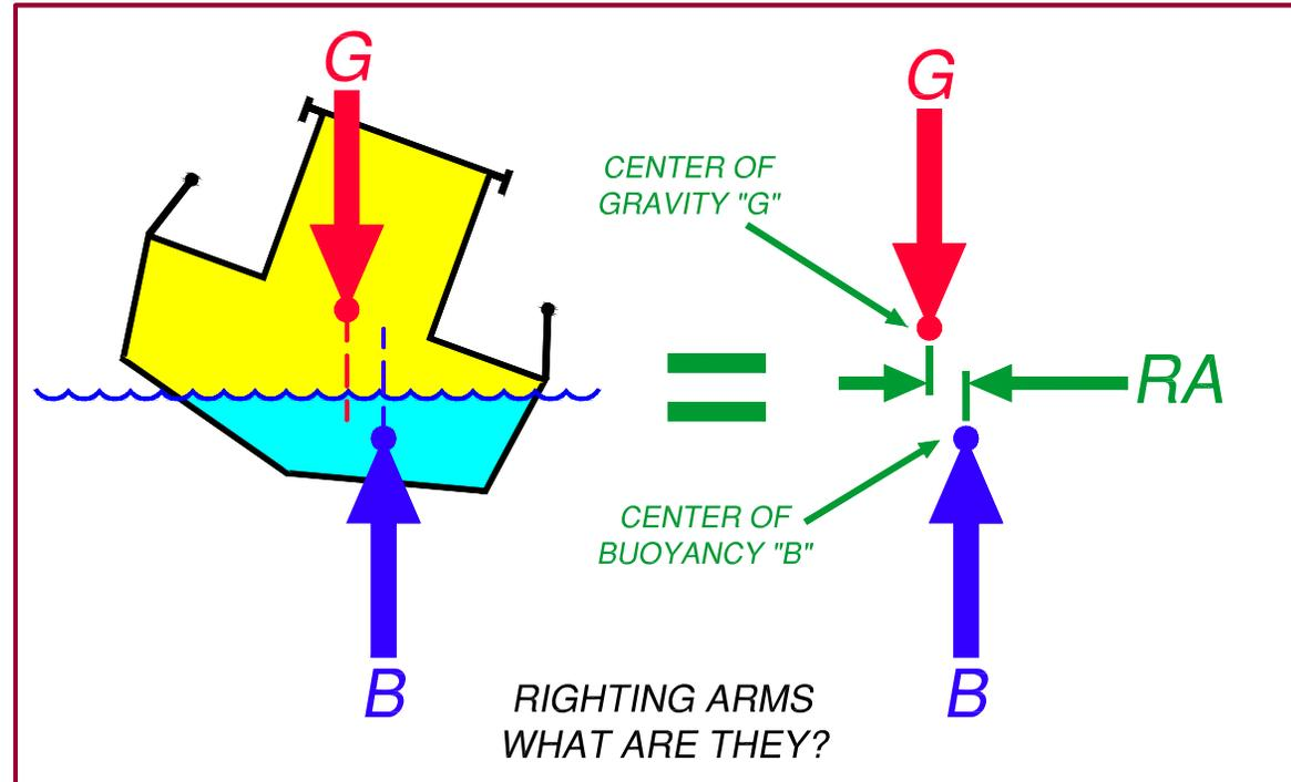
When the center of buoyancy "B" has shifted farther outboard than the center of gravity "G" as shown in the figure, the righting arm "RA" is a positive number creating positive stability.
