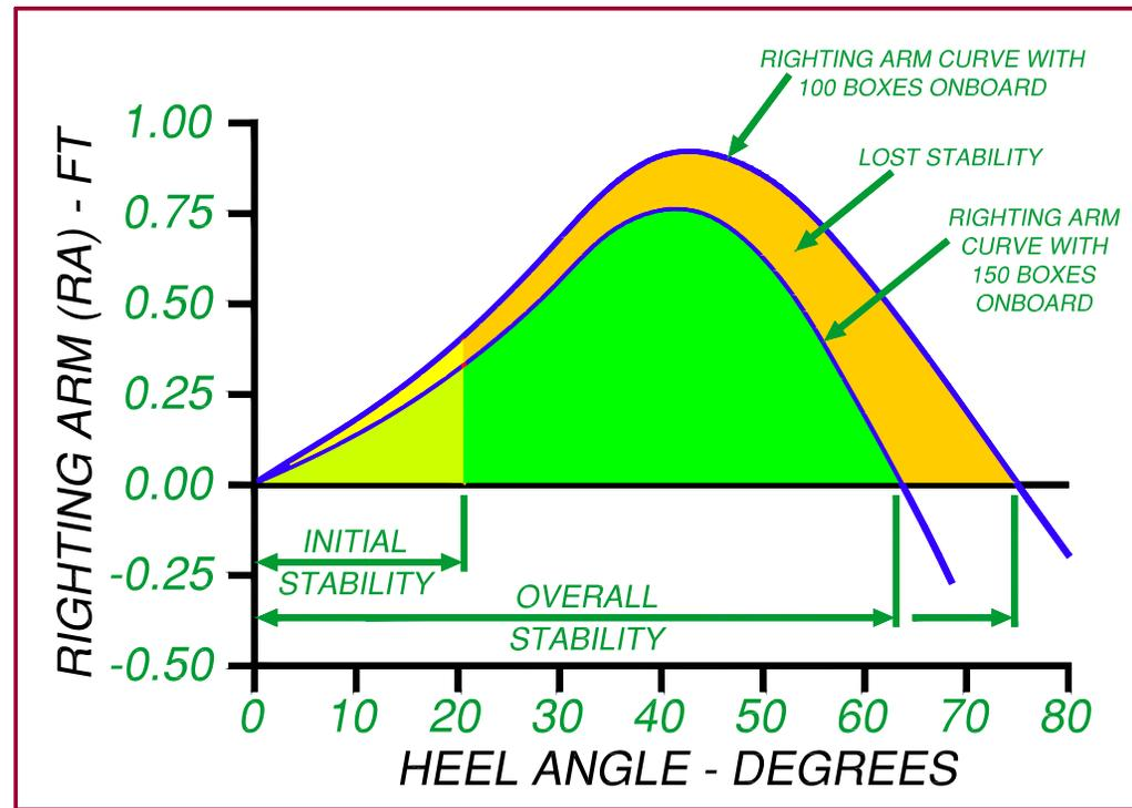
There is a potential hidden danger in using a fishing vessel's "feel" to determine if the vessel is safe from capsizing. The initial stability felt by the crew can be deceiving and give a false impression that the vessel has adequate stability levels. It may be too late to correct a problem by the time the vessel "feels" unsafe.
