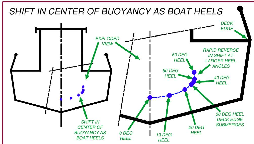
The left diagram shows how the location of a typical fishing vessel’s center of buoyancy shifts outboard as it heels over. Note how the outboard shift reduces when the freeboard deck edge becomes submerged and eventually reverses direction as the vessel heels further.
