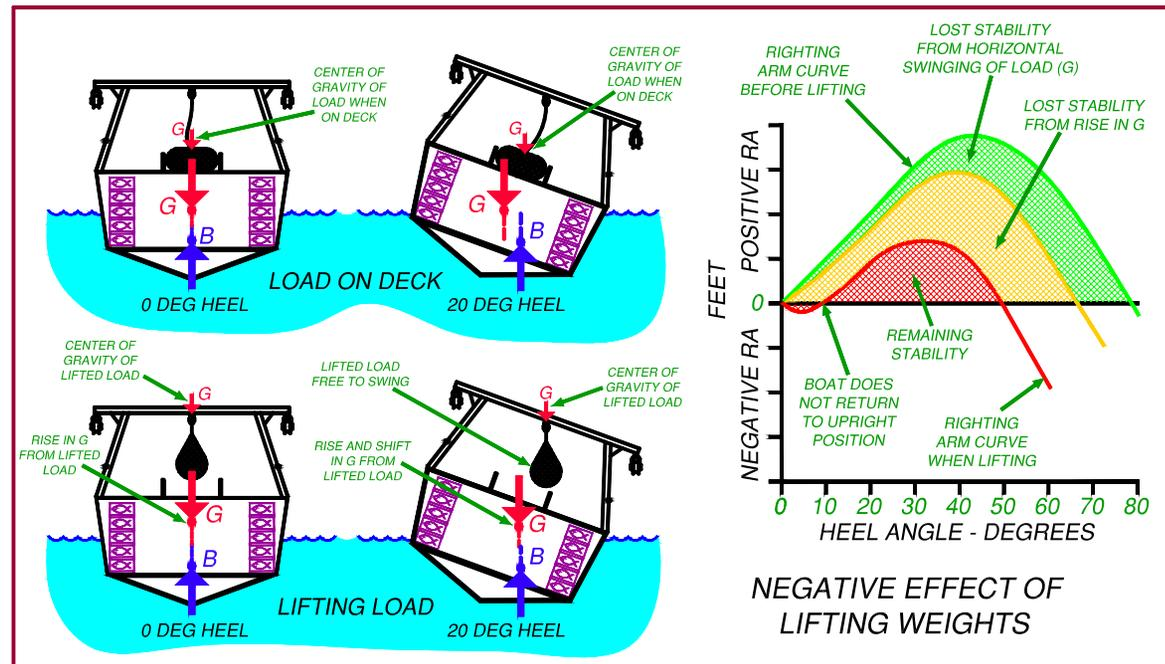
**Recommendations:** Never lift more weight than recommended in the vessel's stability guidance.
