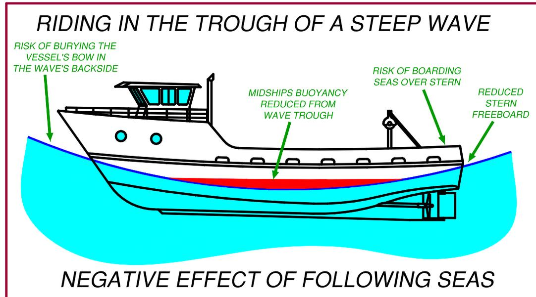
Recommendations: In severe sea conditions, change course to put the bow into the seas. If the vessel must run with the seas, riding on the backside of the preceding wave minimizes the dangers.
