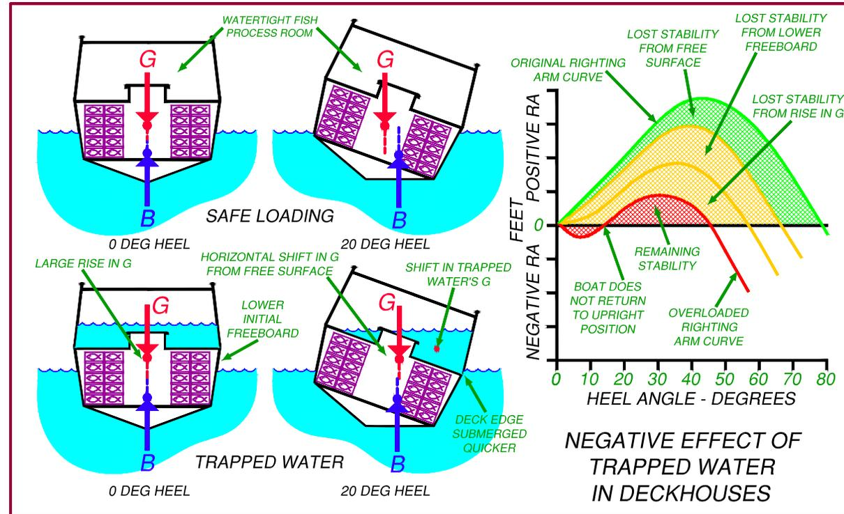
Recommendations: All watertight and weathertight openings should be closed and secured to prevent flooding. In addition all fish processing area drains must be of adequate size and kept clear to prevent any standing water from accumulating in the fish processing area.
