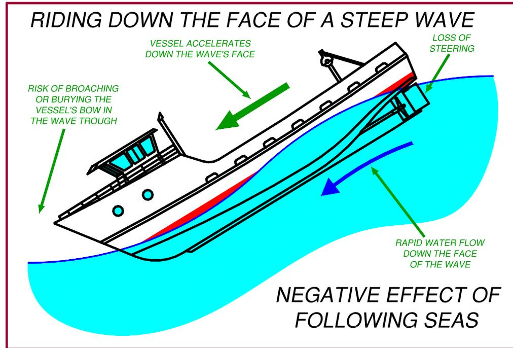
Recommendations: In severe sea conditions, change course to put the bow into the seas. If the vessel must run with the seas, riding on the backside of the preceding wave minimizes the dangers.
