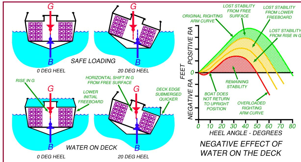
Because the trapped water on deck is located high on the vessel, the fishing vessel may not return to the upright equilibrium condition. Instead, it will lay over or "loll" at the angle of heel where the new righting arm curve goes through zero.
