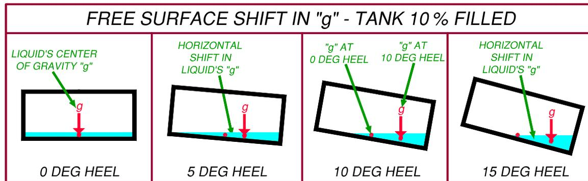
This shift in the liquid's center of gravity "g" causes the vessel's center of gravity "G" to shift outboard, reducing the righting arm "RA" as shown in the figure to the right.
