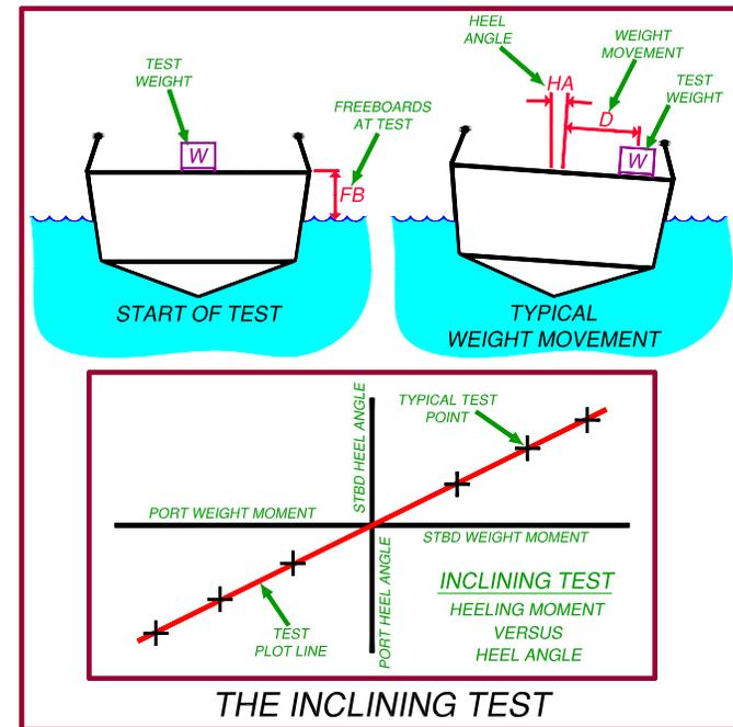
**Preparation of the Vessel:** The vessel should be as complete as possible with all fishing gear onboard. If possible the vessel's tanks should be pressed full or pumped dry to minimize free surface effects (see page 28). In addition all bilges and compartments should be pumped dry.
