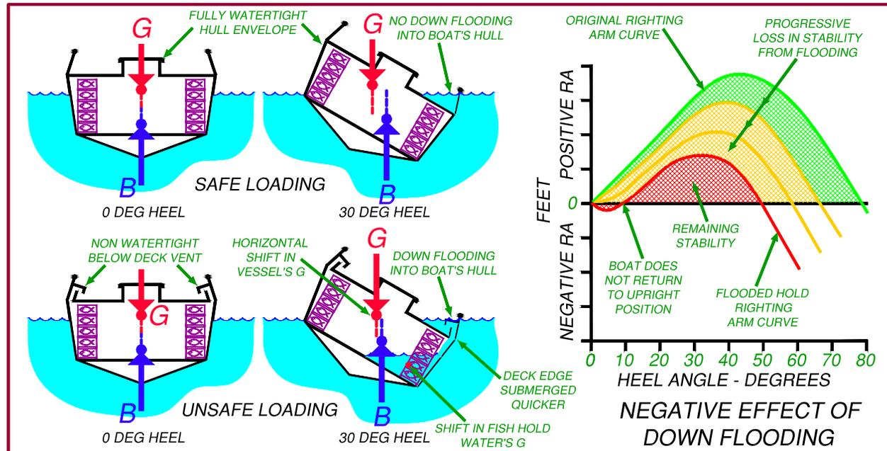
After downflooding occurs, the vessel's overall stability is reduced because:
