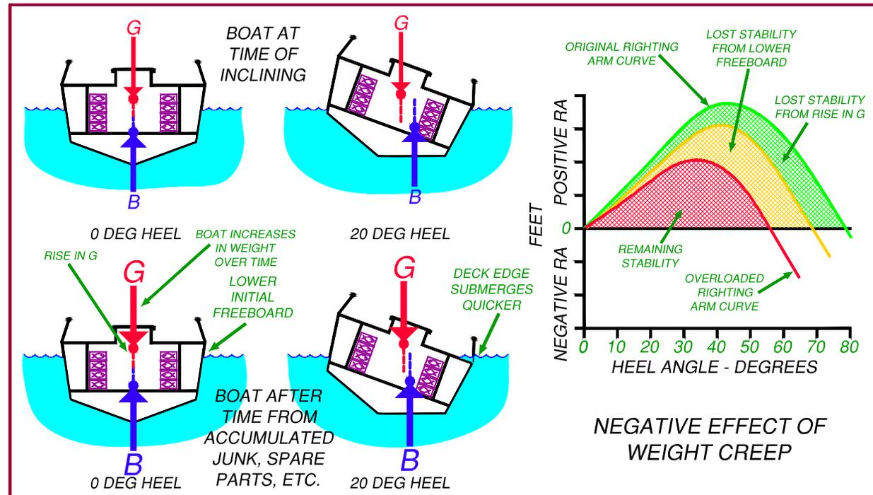
Recommendations: Every 6 to 12 months, all areas of the vessel should be thoroughly inspected and cleaned of any extraneous spare parts, fishing gear, and equipment. If modifications to the vessel or its fishing gear not included in the vessel's current stability assessment must remain, consult a Naval Architect about developing new stability guidance.
