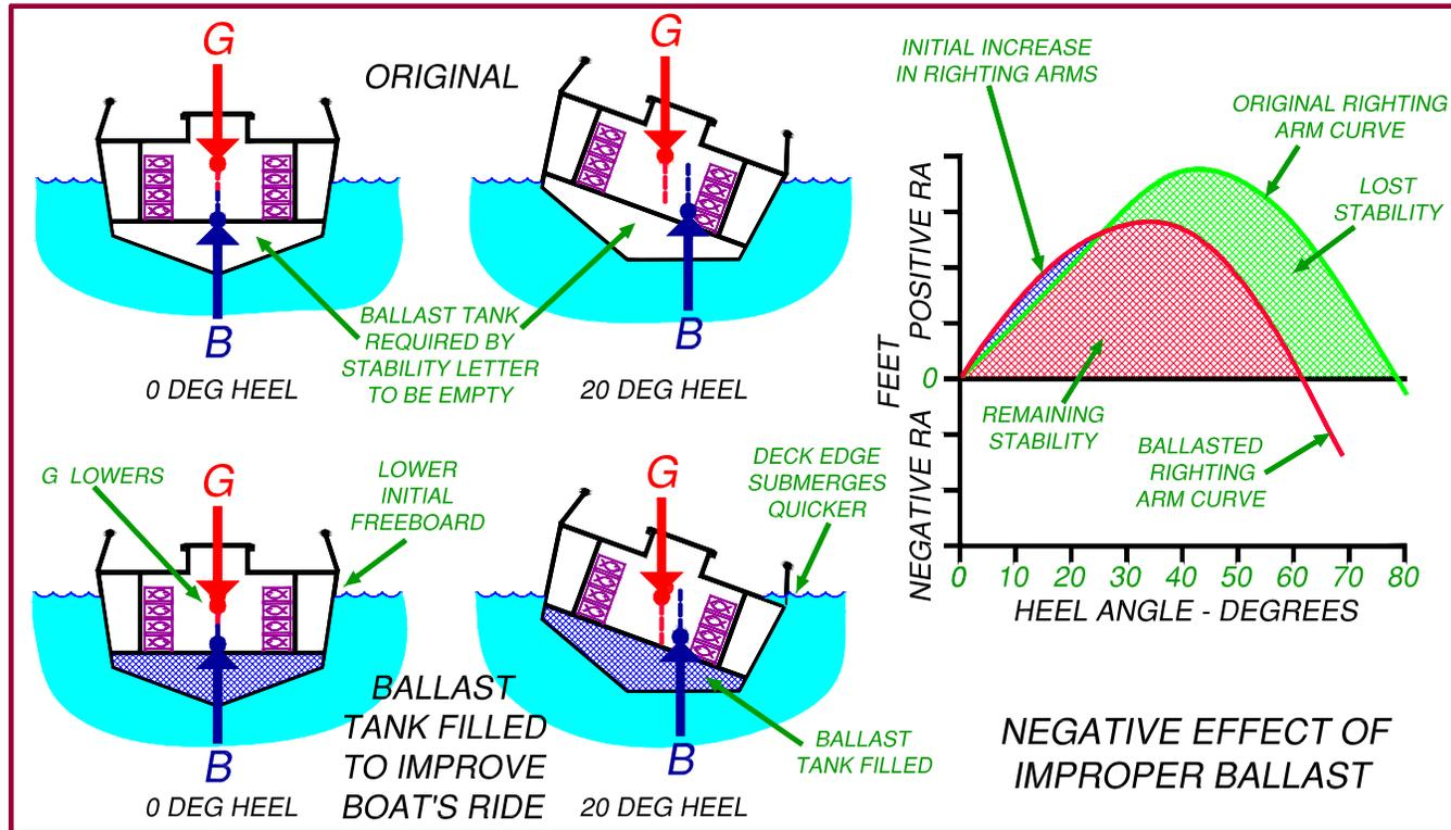
The vessel's overall stability though has been downgraded because the freeboard is reduced, causing the freeboard deck edge to submerge at smaller heel angles.
