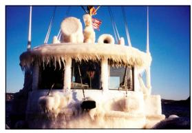
If you encounter severe Ice Accumulation, you should head to port immediately, if possible. If your vessel is not able to make it to port, head for the lee of an island, if available. The island will block some of the wind and waves. In the lee of an island, maneuver your vessel so that you take the wind and waves on the stern to reduce the spray created by the vessel. If you are unable to find shelter, maneuver your vessel so that you minimize the spray created.
