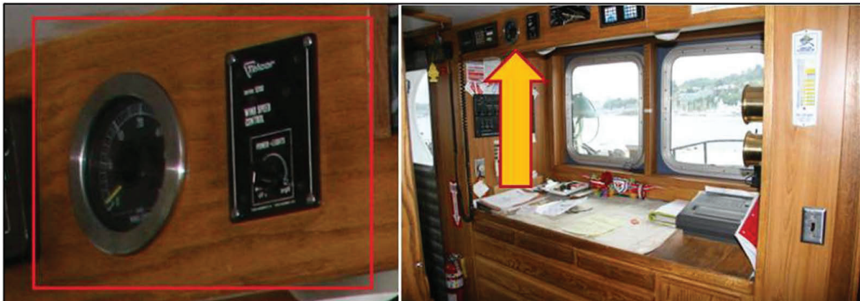
Figure 40 – Wind speed indicator with controller mounted on the upper part of the after-wheelhouse bulkhead of the SCANDIES ROSE that indicate apparent wind speed in knots. The device does not measure wind direction. Also shown in the bottom right of the right picture is the weatherfax, another means to receive weather information. (Source Captain [redacted] Survey Photos)
