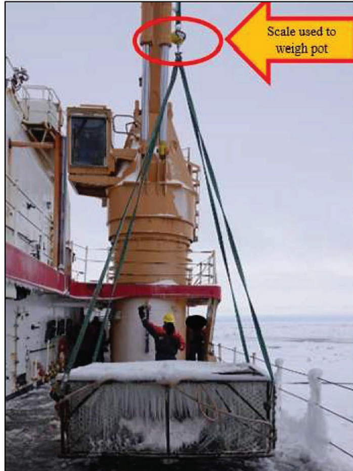
Figure 118 – The crab pot that was subjected to the freezing freshwater spray is weighed onboard the POLAR STAR at the conclusion of a 72-hour period. The yellow arrow points to the scale mounted in the lifting apparatus. (Source Coast Guard)
