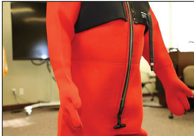
Figure 102 – SCANDIES ROSE survival or immersion suit showing the three-finger glove which is attached to the neoprene arm of the suit. The three-finger glove protects the hand from hypothermia but compromises manual dexterity for tasks like opening buckles or activating flares. (Source CG Exhibit 103)
