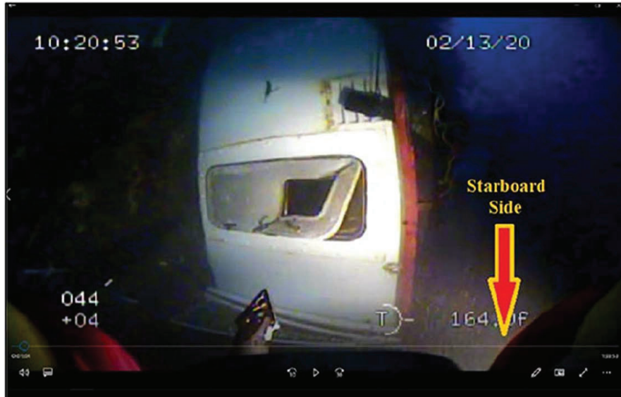
Figure 25 – After starboard side accommodation door of the SCANDIES ROSE on the after bulkhead showing damage. (CG Exhibit 008, with markup)
