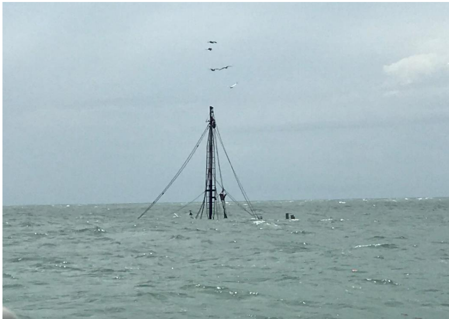
Figure 4. The LADY DAMARIS after capsizing on the starboard side, with the port outrigger exposed above water.
