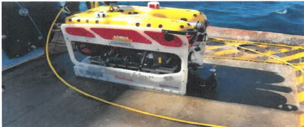
Figure 43: Saab SeaEye Falcon DR ROV. Image courtesy of WHOI, 2021.
