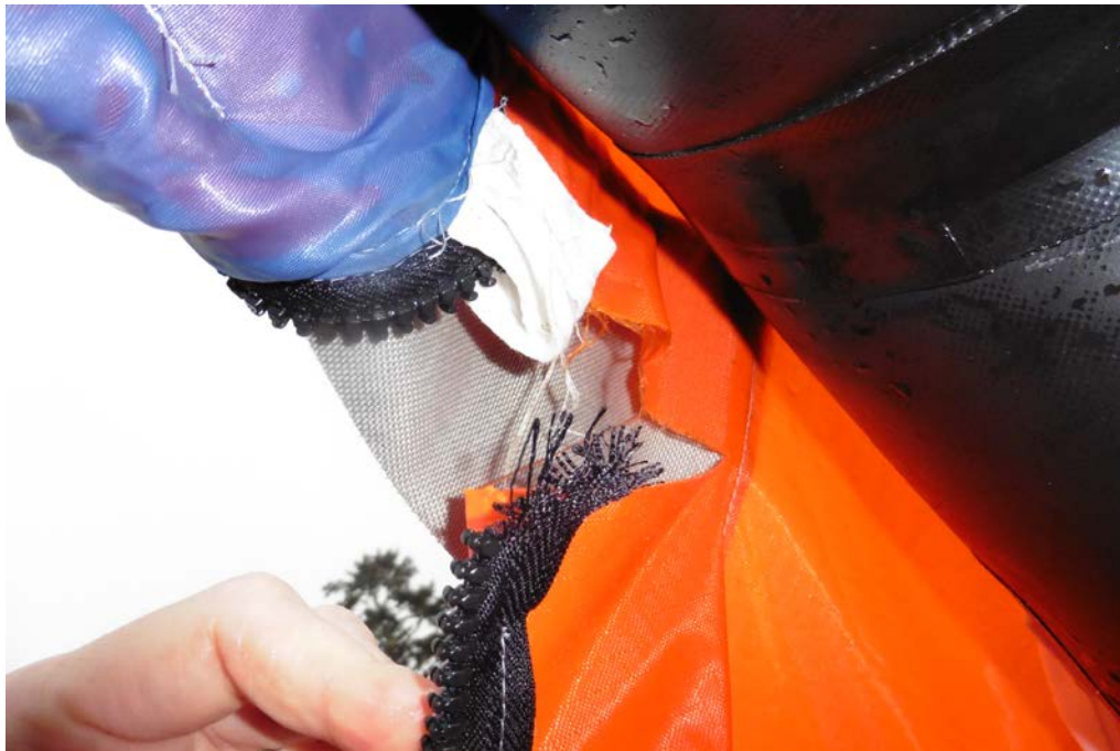
Figure 8: Photo of tear in life raft canopy entrance flap.
