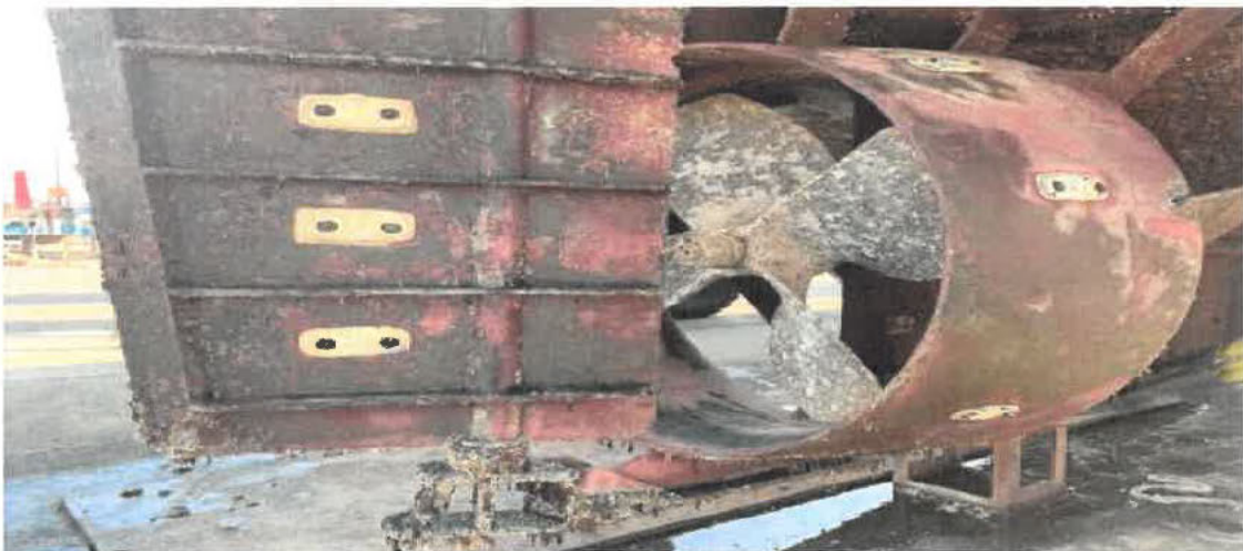
Figure 71: Skeg hung steering and propulsion gear of the EMMY ROSE, Image courtesy of Marine Safety Consultants.
