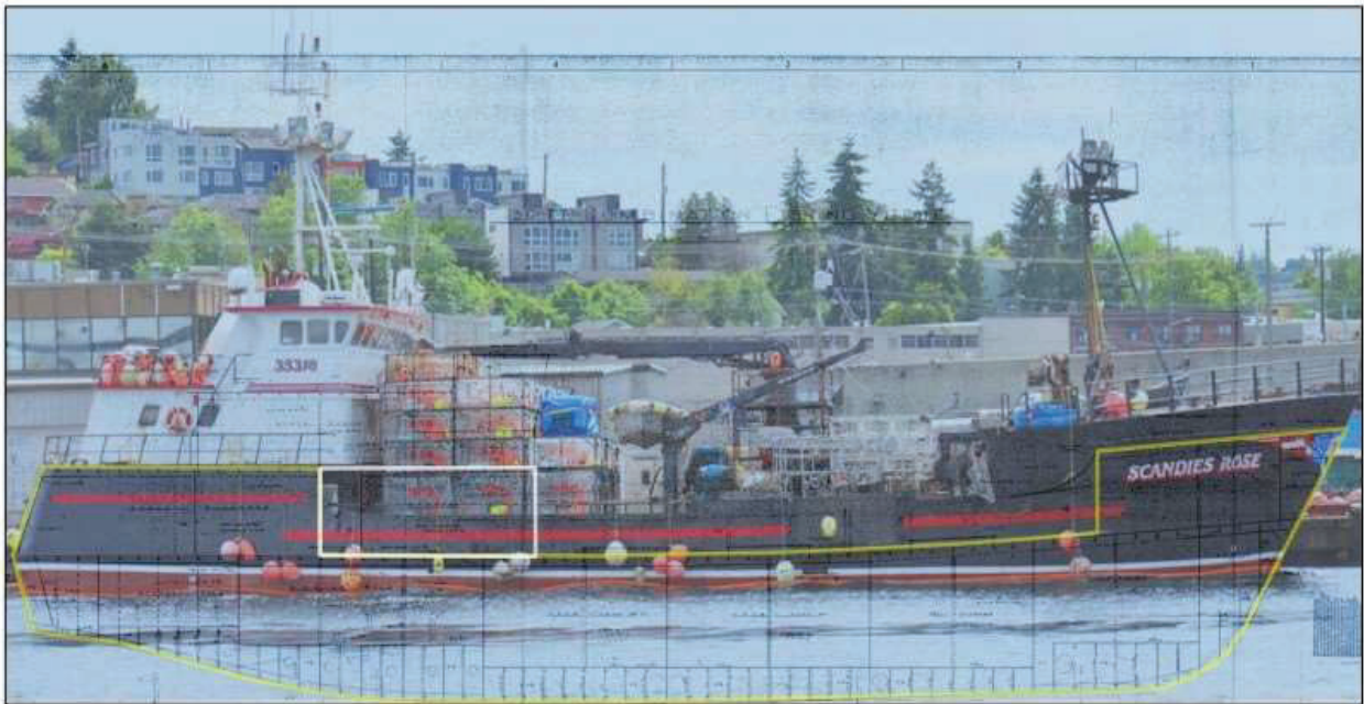
Figure 51 - Profile photograph of the SCANDIES ROSE with Scantling Plan and Profile overlaid. Note that the plan matches the vessel's transom but indicates additional buoyant volume at the forward end of the poop. (White highlighted area) (Source USCg MSC Report, CG Exhibit 059)
