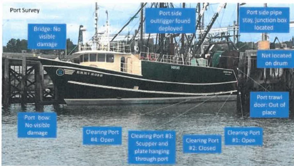
Figure 69: Port side ROV survey results of the EMMY ROSE. Image courtesy of WHOI, 2021.
