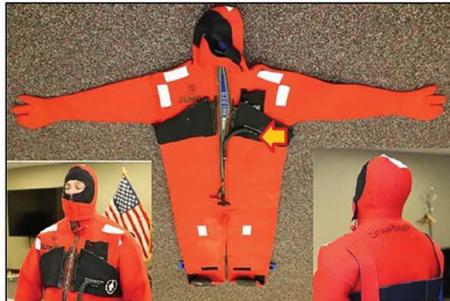
Figure 101 - Composite of photos of one of the survivor's actual survival or immersion suit. The yellow arrow indicates the manual inflation tube for inflating the bladder to assist upright floatation. Mr. [REDACTED] is wearing the suit in this demonstration. (Source CG Exhibit 103 composite with mark ups)
