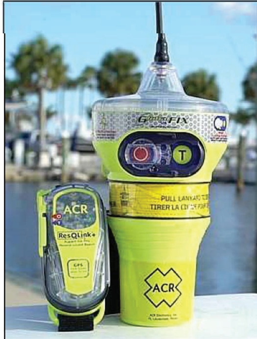
Figure 104 – On the left, is an ACR Electronics Inc. version of a PLB that could have been carried by the crewmembers on the vessel. On the right of the same image is an EPIRB of the type and manufacture that was carried on the SCANDIES ROSE. The figure gives a perspective as to the size of the devices in comparison to one another. (Source Coast Guard)
