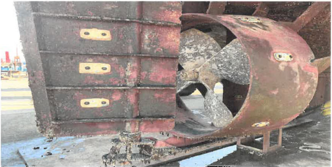
Figure 28: EMMY ROSE running gear. Image courtesy of Marine Safety Consultants, 2019
