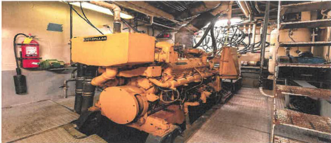
Figure 25: EMMY ROSE Maine Diesel Engine, looking aft. Image courtesy of Atlantic Brokerage.
