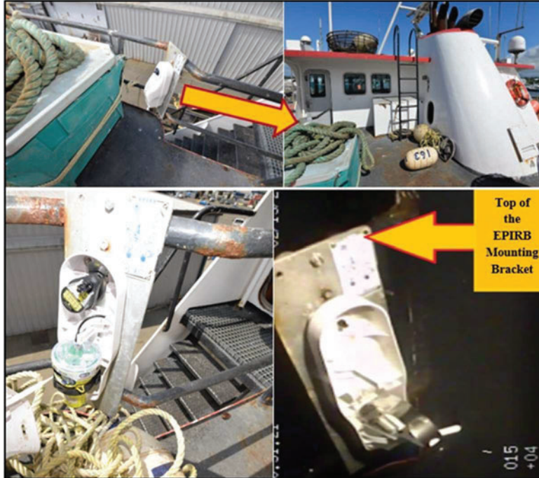
Figure 14 – Composite of photo montage of the SCANDIES ROSE EPIRB. Top left, EPIRB in housing on the inside of top rail aft of the wheelhouse. Top right is the location shown with the yellow arrow in reference to the position in relationship to the port wheelhouse door. Bottom left, the open EPIRB housing during inspection for 2019 Valuation and Condition Survey. Bottom right, the empty housing as seen during underwater site survey conducted by Remotely Operated Vehicle (ROV) in February 2020. (Source – [REDACTED] photos for 2019 Valuation Survey and bottom right, CG Exhibit 008)
