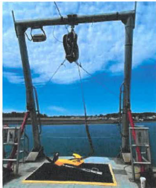
Figure 37: Klein 4000, primary side scan sonar used for search for EMMY ROSE. Imagery courtesy of MIND Technologies.
