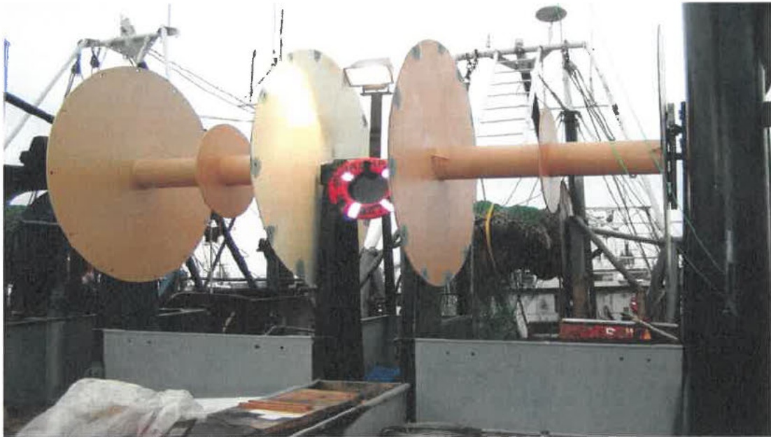
Figure 8: Net reels added to the SASHA LEE in 2001. Image courtesy of Thomas M. Farrell Naval Architects.
