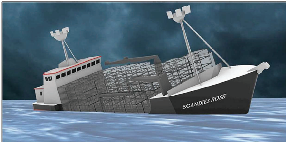
Figure 10 - SCANDIES ROSE Marine Safety Center (MSC) modeling with a 20-degree list to starboard as described in section 4.1.34.2. of the ROI. (Source Coast Guard Marine Safety Center)
