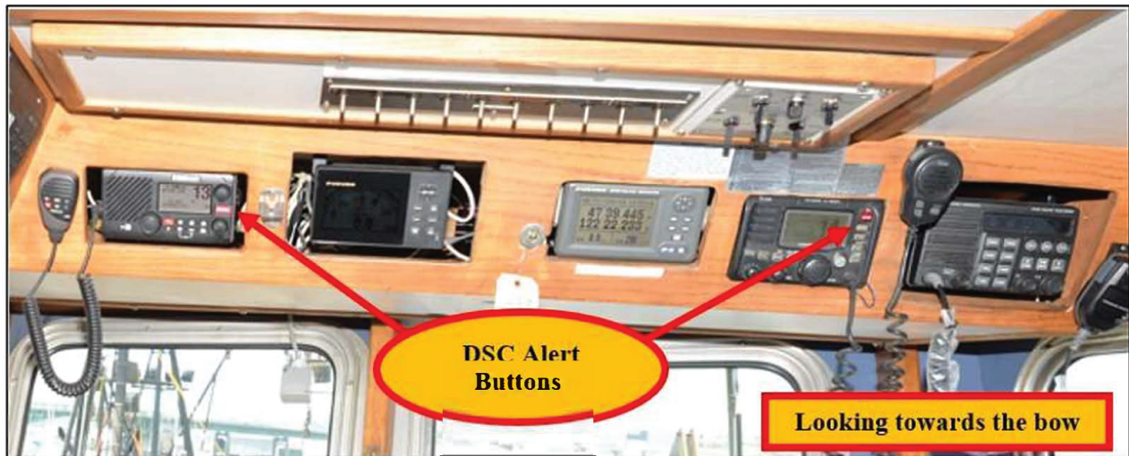
Figure 105 – Marine VHF radios above the starboard control station on the SCANDIES ROSE. The red arrows indicate the location of the DSC buttons on each radio. Each radio was manufactured with the DSC feature built in, but there is no evidence that this feature was properly configured with MMSI number and GPS input for use in an emergency. (Source CG Exhibit 004, with mark ups)
