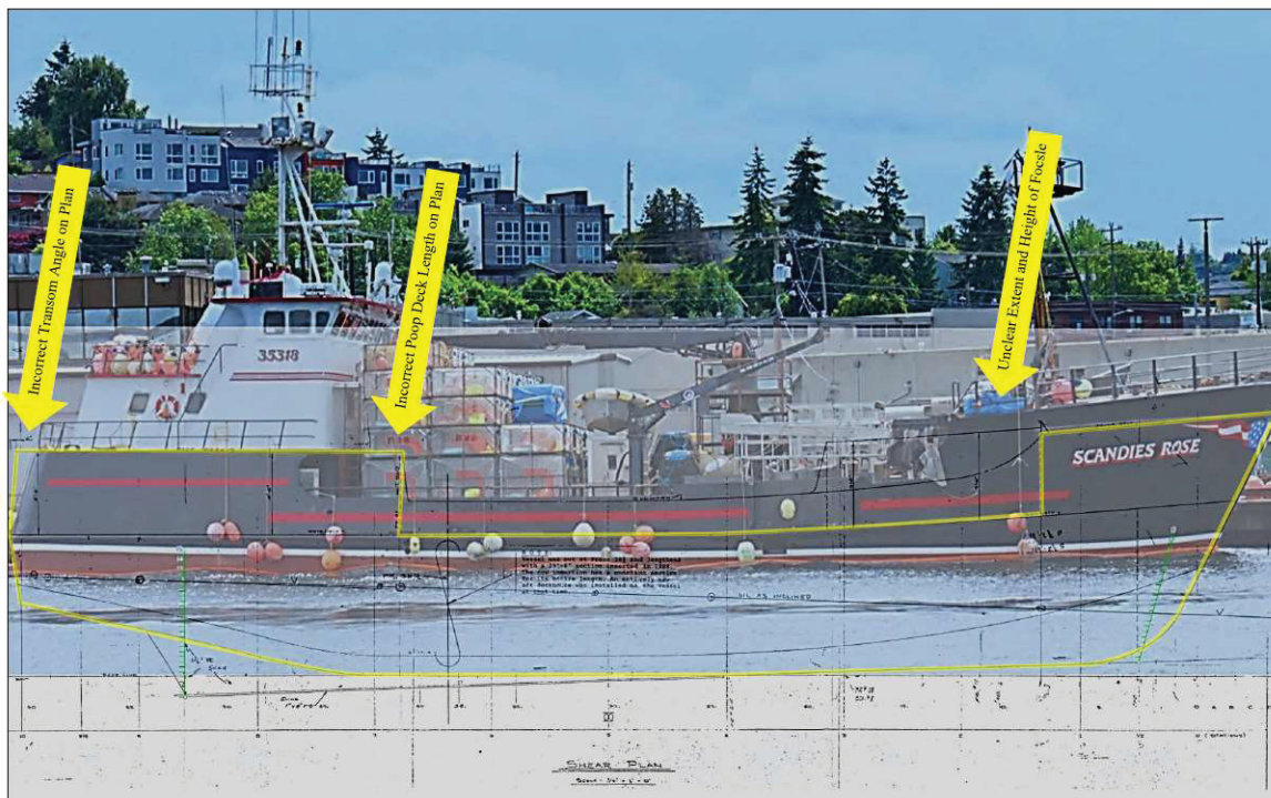
Figure 81 – 2019 Profile photograph of SCANDIES ROSE with Lines Plan profile overlaid with watertight envelope highlighted in yellow and large profile differences in the poop and forecastle called out. (CG Exhibit 059, Pg. 9)
