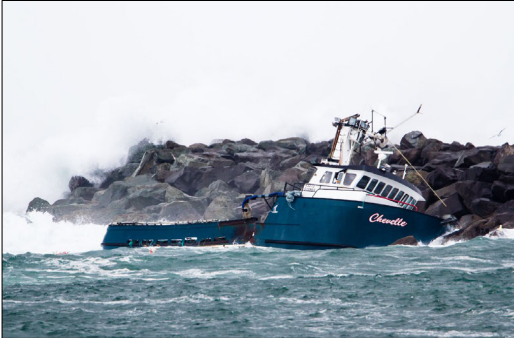
Figure 39. Image above demonstrates the danger posed by the breaking bars at the North Jetty of the Yaquina Bay Bar near the north tip. Note the large size and placement of the rocks used to form the protective jetty. The F/V CHEVELLE accident occurred in March 2012, the vessel was a total loss and all crew were recovered safely. (Photo - Mr. and Mrs. [REDACTED] ©)
