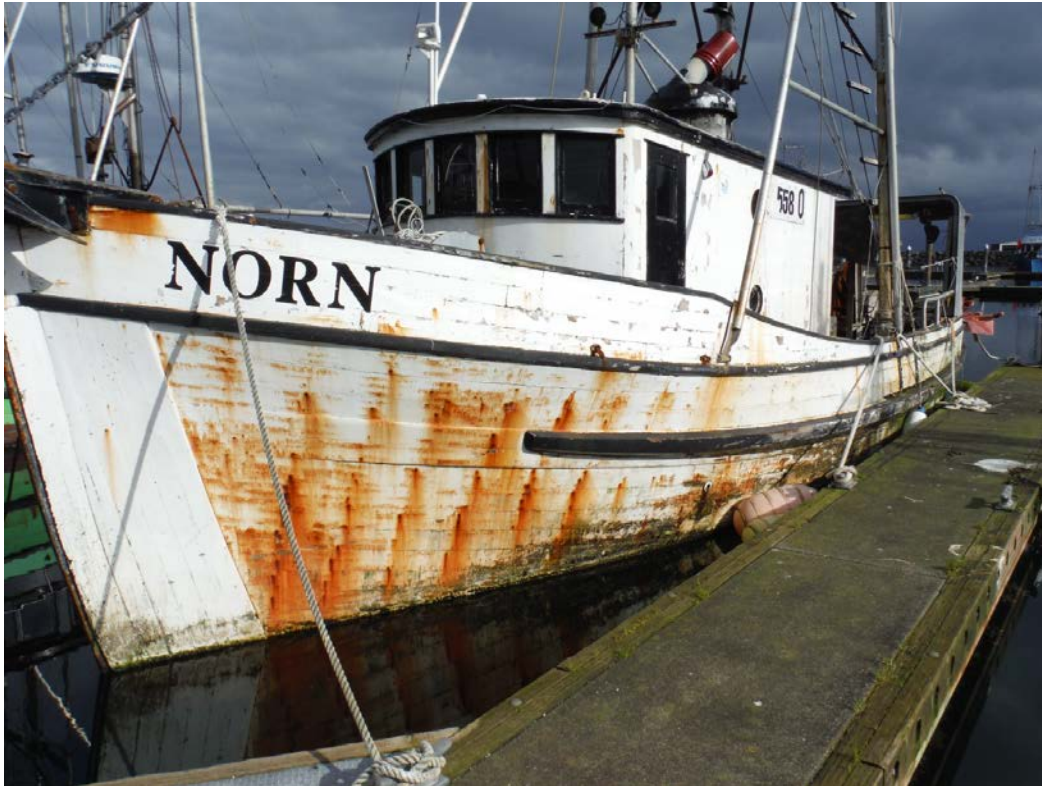
Figure 10: NORN's port bow. Picture taken March 2013. Bleeding fasteners are easily visible.
