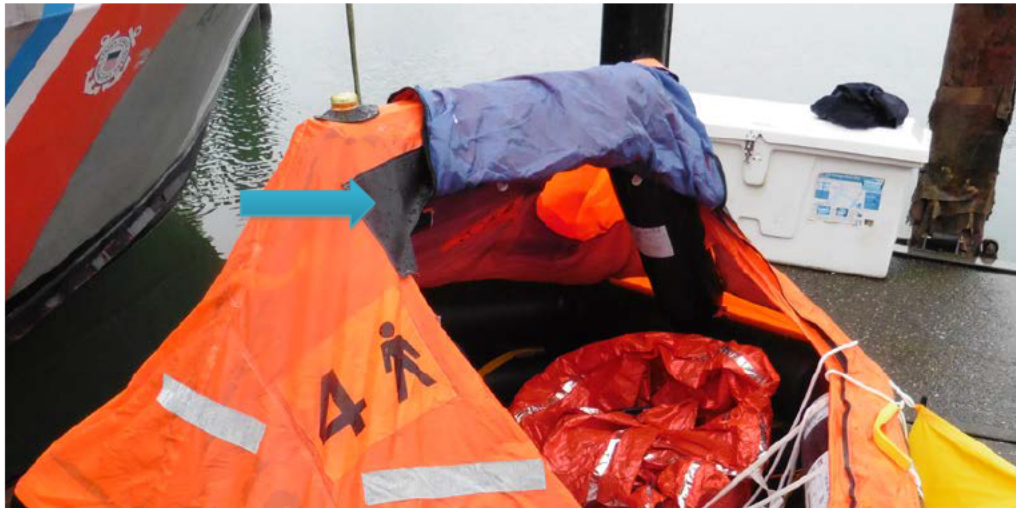
Figure 9: Photo of NORN's life raft. Arrow points to location of flap tear on opposite side.
