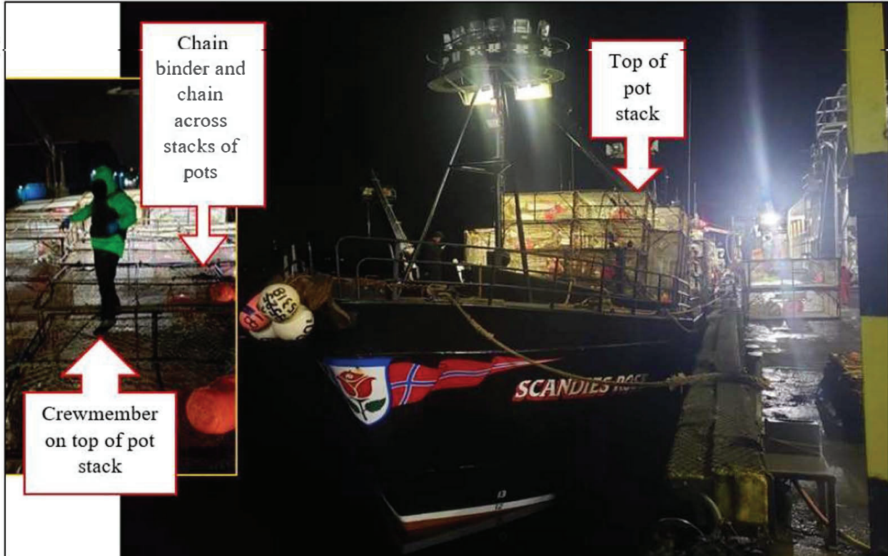
Figure 58 – SCANDIES ROSE at the dock just prior to departure with chain binders, chains and height of the pot stack at its highest point shown. (Source Mr. [REDACTED] and Mr. [REDACTED])
