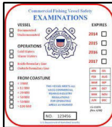
Figure 22. A sample of a CFV Safety Decal which would be issued to a vessel after it has been inspected by qualified Coast Guard Fishing Vessel Examiners and found to be in compliance with the requirements of 46 CFR § 28. (Source – Coast Guard)
