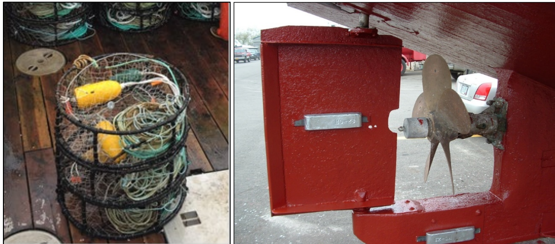
Figure 56. (Left) Image of crab pots and lines associated with the use of these pots, showing the general type of line that may have fouled the propeller, rudder or propeller shaft of the MARY B II to an unknown degree. (Source – Coast Guard). (Right) Underwater aft section of the
