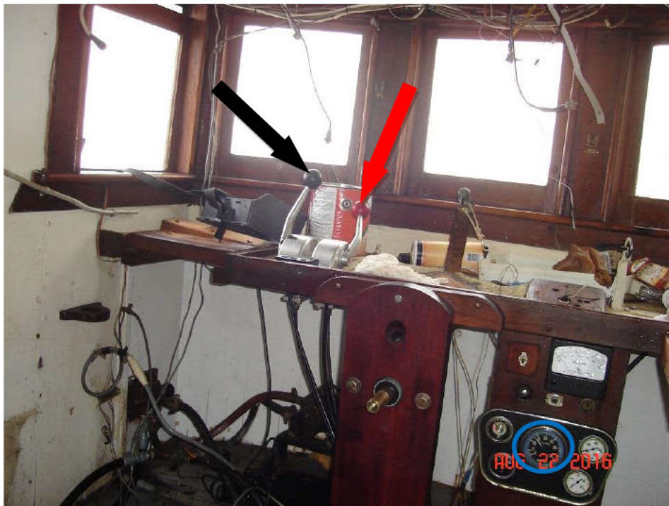
August 22nd photo of the wheelhouse of the ILA showing engine controls (gear control indicated by black arrow; throttle indicated by red arrow) and engine tachometer (circled in blue at lower right).
