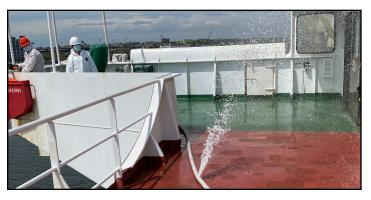
able to deliver the required two jets of water due to malfunctioning impellers. The ship had to run both pumps simultaneously to supply enough pressure. Finally, despite only two issues related to inoperable smoke detectors, there were still a few deficiencies related to smoke detectors being found covered with plastic bags.
