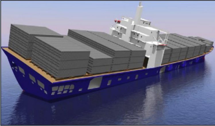
EL FARO computer model with a 15 degree starboard list and 5.8 ft of trim by the stern. MSC calculated that hold 3 was flooded to 20 percent.
