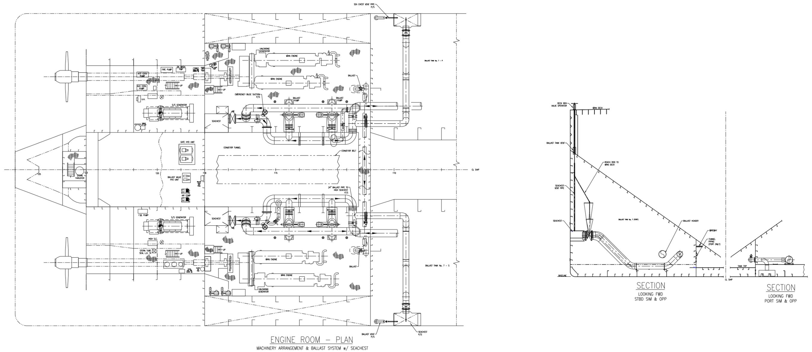
Figure B-3. Large capacity 1000' Laker: engine room arrangement.
