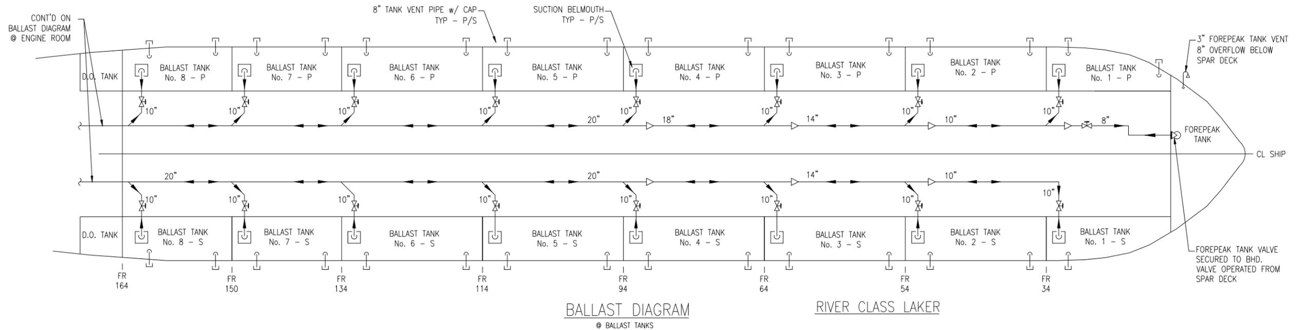
Figure E-4. Small capacity, river class 600' - 700' Laker: ballast diagram.
