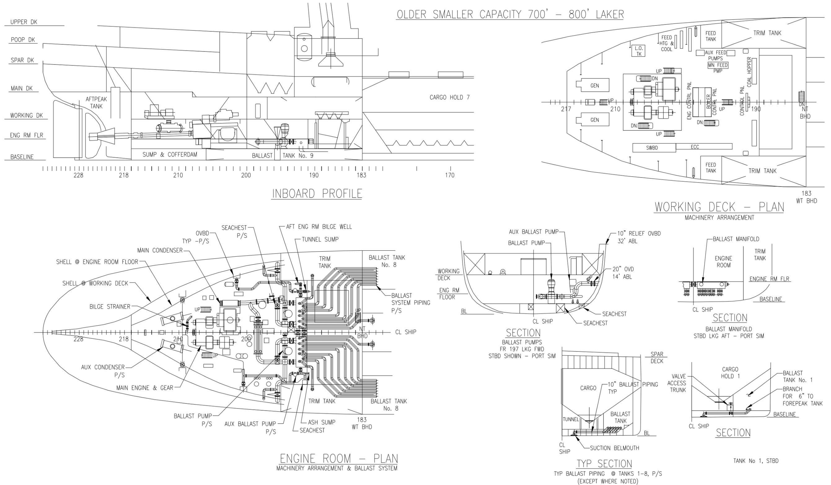
Figure C-3. Older, small capacity 700' - 800' Laker: engine room arrangement.
