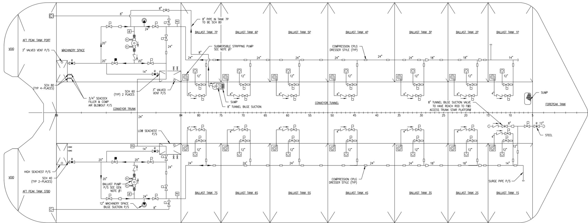
Figure D-4. Newer, intermediate capacity 800' – 900' Laker: ballast water diagram.
