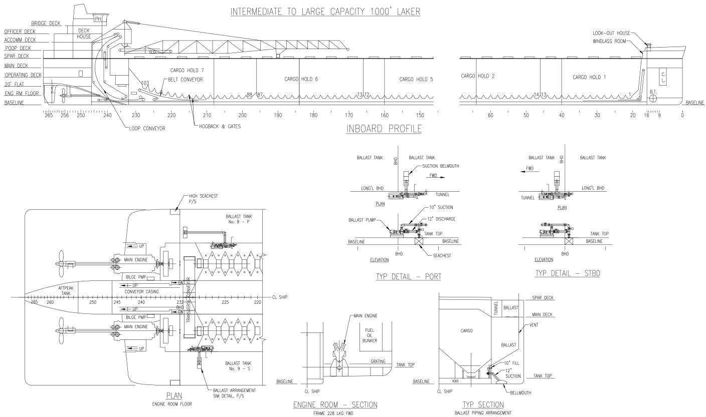
Figure A-3. Intermediate to large capacity 1000' Laker: engine room arrangement.
