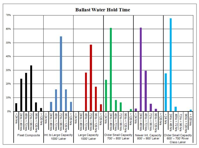
Figure 6. Ballast water hold time.
