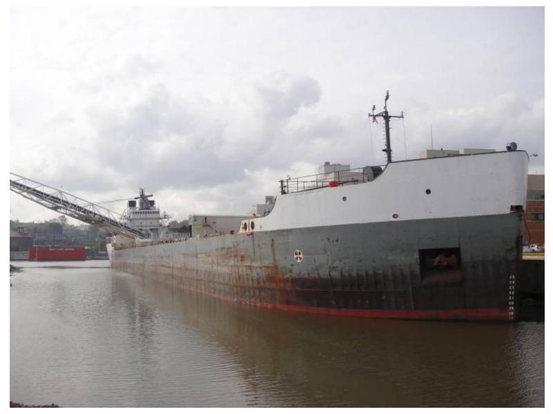
Figure E-1. Small capacity, river class 600' – 700' Laker: photo.
