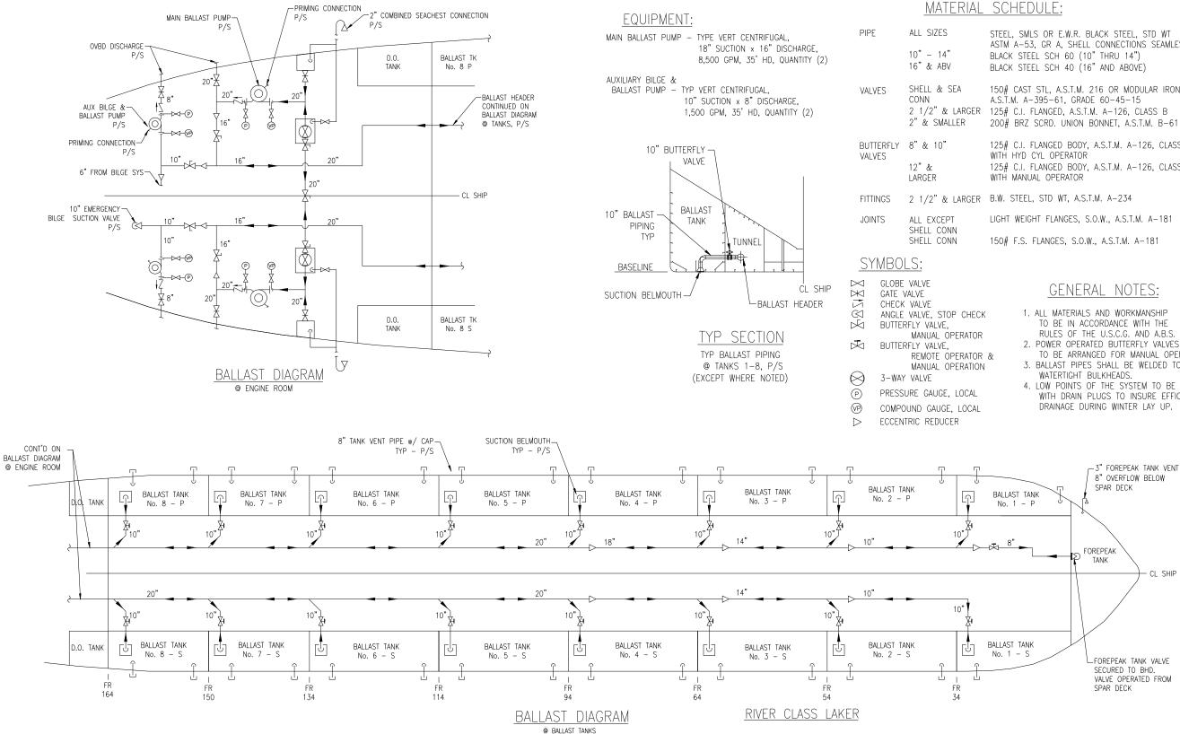
Figure E-4. Small capacity, river class 600' - 700' Laker: ballast diagram.
