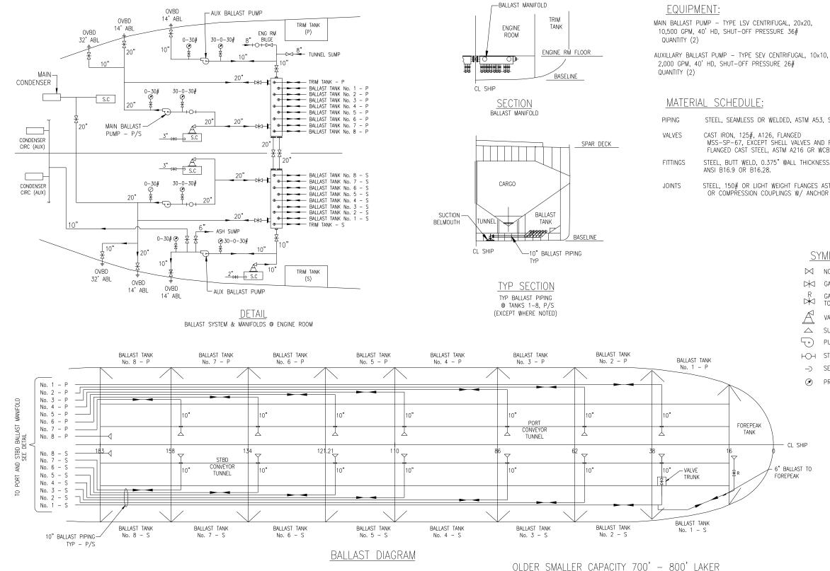
Figure C-4. Older, small capacity 700' - 800' Laker: ballast diagram.
