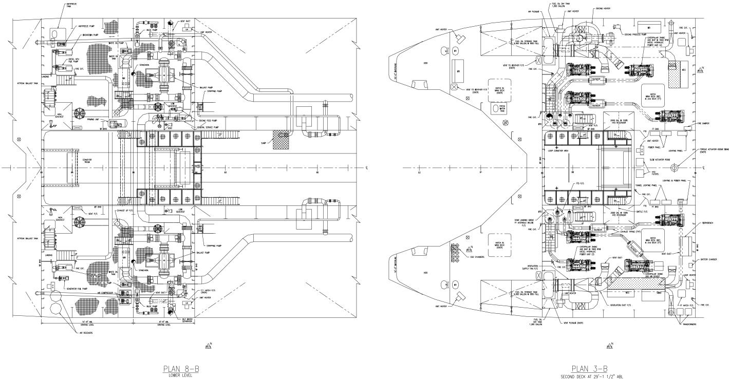
Figure D-3. Newer, intermediate capacity 800' – 900' Laker: engine room arrangement.
