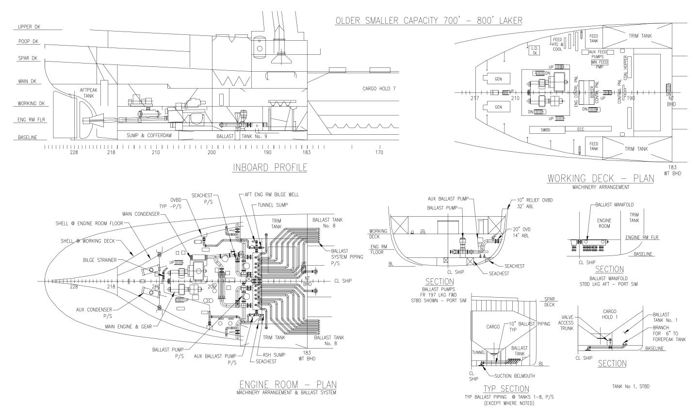
Figure C-3. Older, small capacity 700' - 800' Laker: engine room arrangement.
