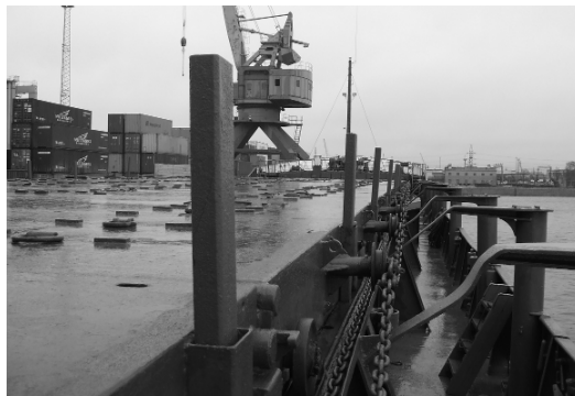
Figure 6.7. Example of uprights for bottom blocking
