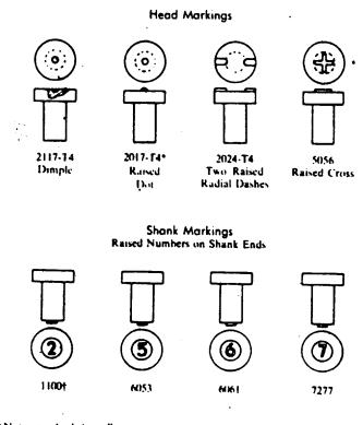
\* Not a standard rivet alloy. †1100 not marked unless so specified.
