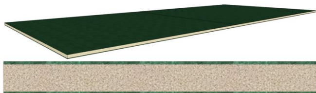
Figure 1: Illustrations of a FRP composite sandwich panel composition
