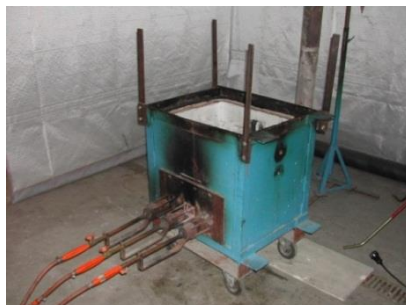
Figure 15: Small-scale furnace for structural resistance tests
