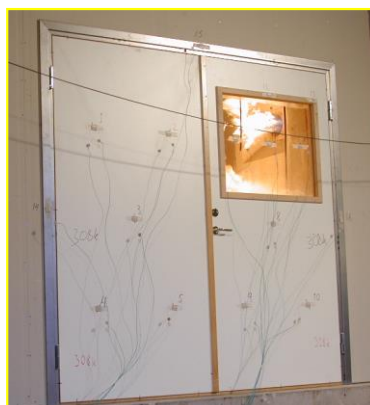
Figure 14: Insulation test of a door where thermocouples measure the backside temperature during the heat exposure
