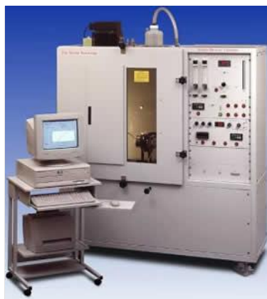
Figure 11: Smoke box equipment
