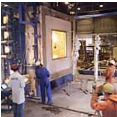
Figure 13: Large scale structural fire resistance test of a window
