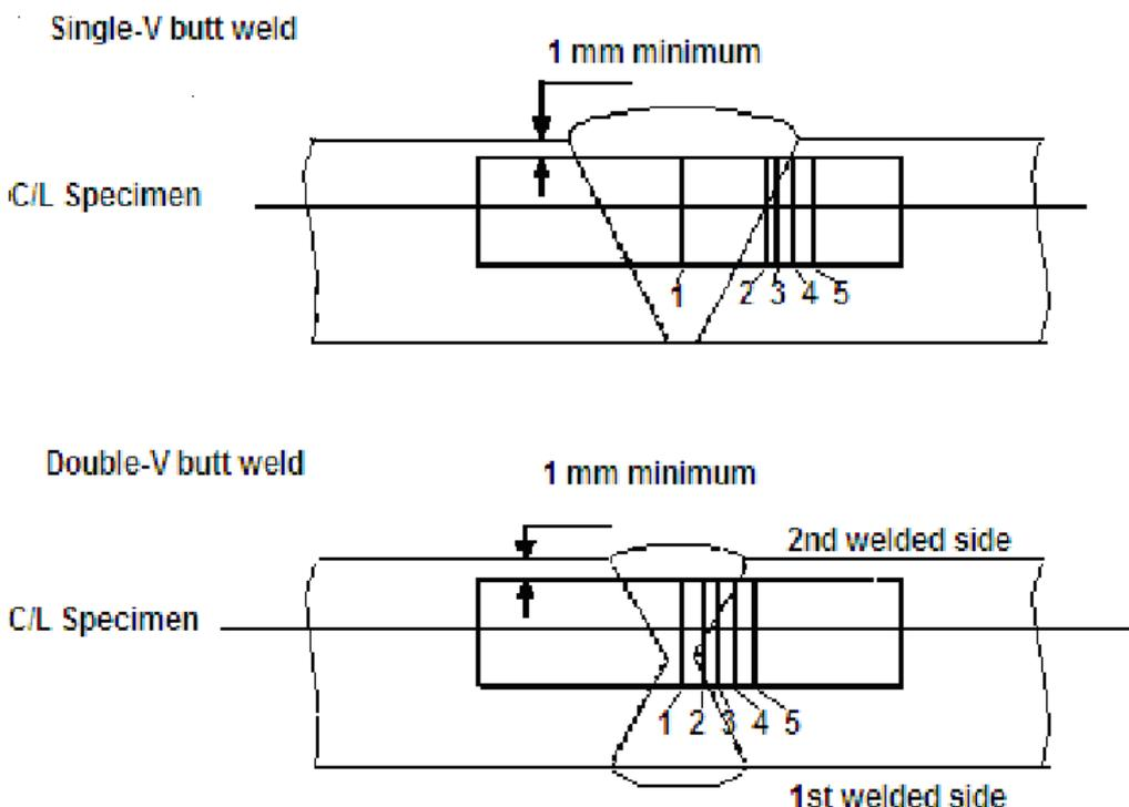
Figure 6.2 – Orientation of weld test specimen
