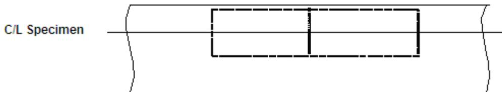
Figure 6.1 – Orientation of base metal test specimen
