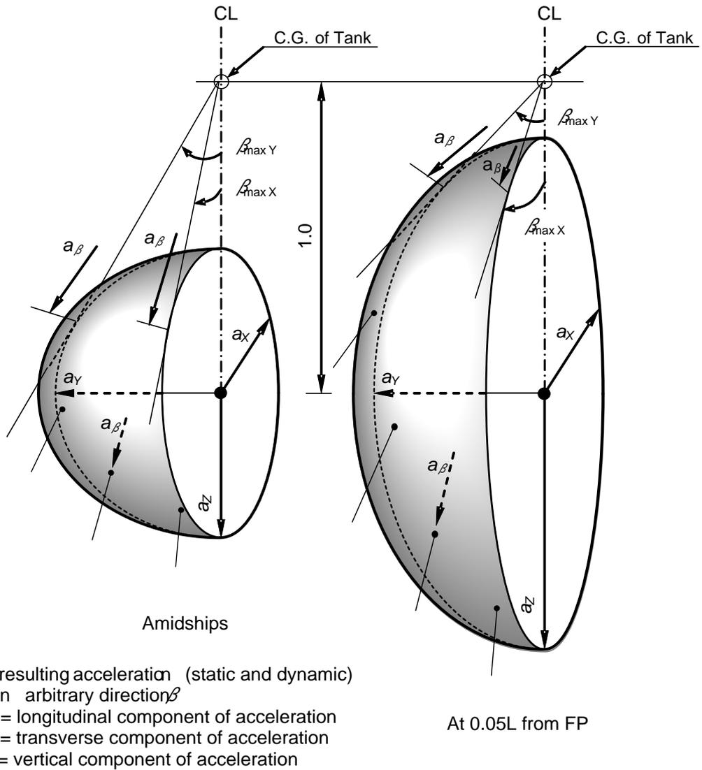
**Figure 4.1 – Acceleration ellipsoid**
