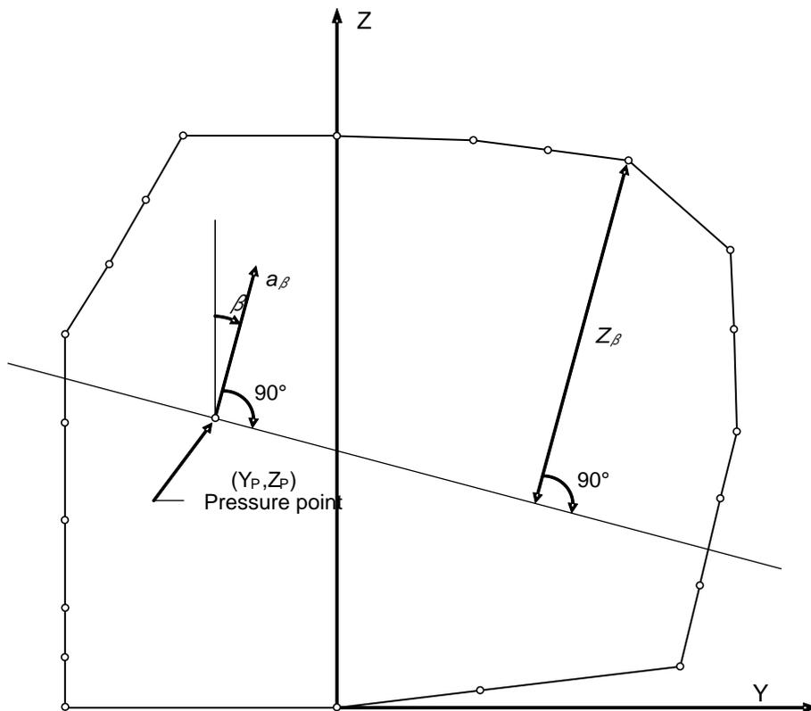
Figure 4.2 – Determination of internal pressure heads
