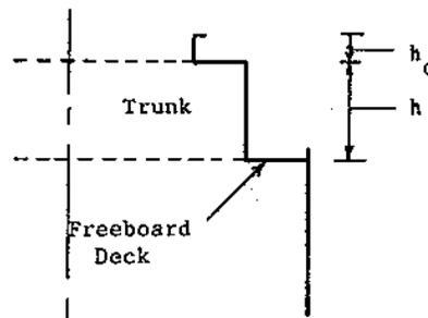
$$\text{Height of trunk} = h + h_c - h_{rc}$$
