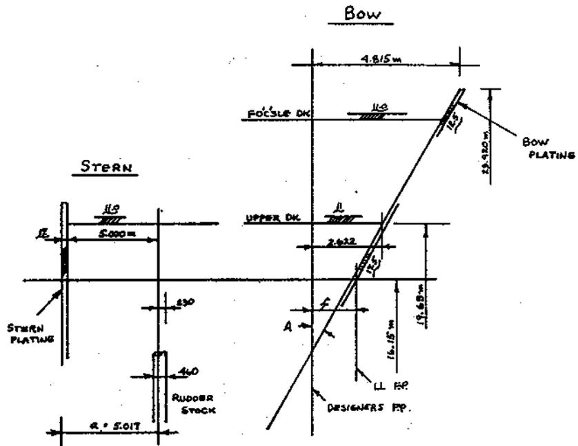
Figure 70. Tanker Load Line Length
