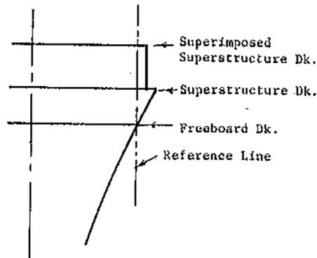
Cross Section at Midlength of Superimposed Superstructure.
