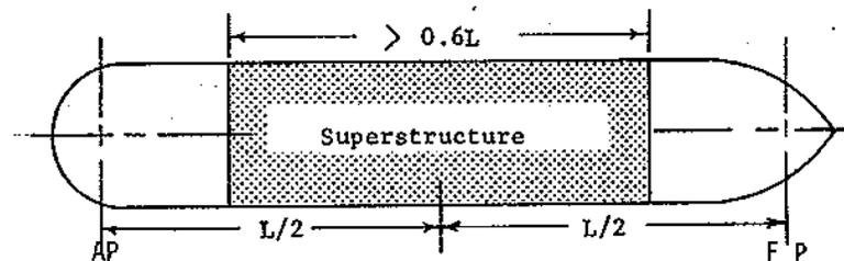
Figure 18. Enclosed Superstructure for Negative Depth Correction Credit
