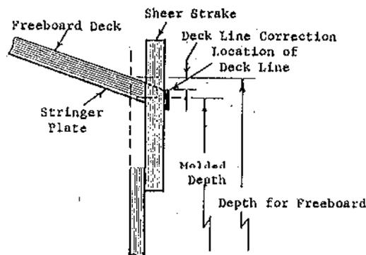
Figure 19. Deck Line Correction
