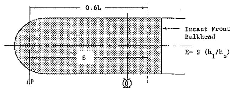
If a raised quarter deck is set in from the side of the vessel for part of its length<sup>27</sup>, the effective length is determined in the same manner as any other superstructure type *except*:
