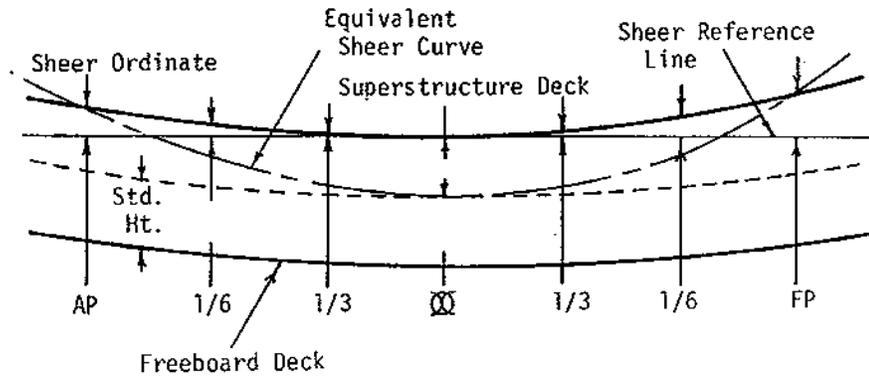
In vessels with a superstructure that extends over the entire freeboard deck that is *less* than standard height, the sheer ordinates are measured at the freeboard deck.
