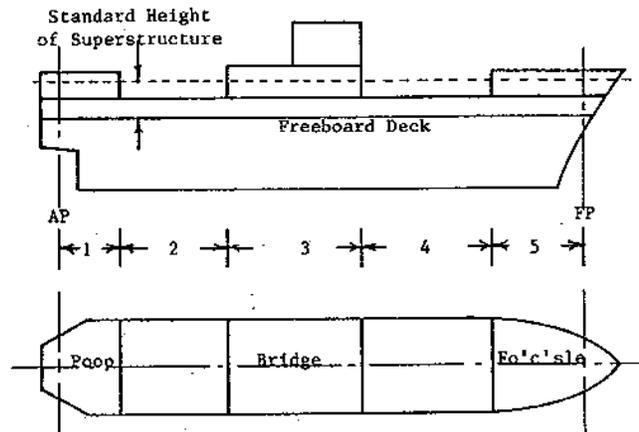
The vessel is divided up into segments that are less than, and greater than standard height. Credit is given for segments 1, 3 and 5 without a height correction. The effective lengths of segments 2 and 4 are adjusted for the height deficiency. The respective effective length of each segment is added to determine the total effective length of the superstructure.
