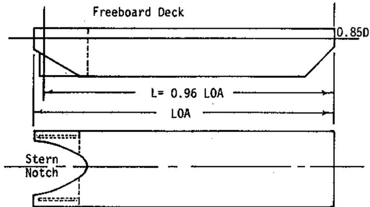
Figure 63. Stern Notch-Load Line Length
