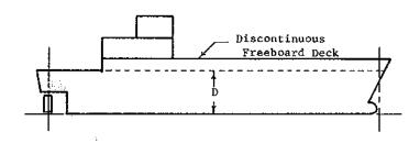
Where a step in the deck to be considered as the freeboard deck, i.e. a discontinuation extending over the full breadth of the ship, is in excess of 1m (3.28 ft.) in length, the lower point of the stepped deck will govern the molded depth, and hence will become the freeboard deck location.<sup>2</sup>
