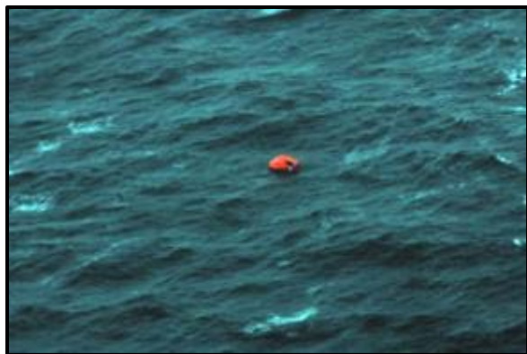
Liferaft in the water. Contrasting color helps SAR facilities locate persons in distress.
