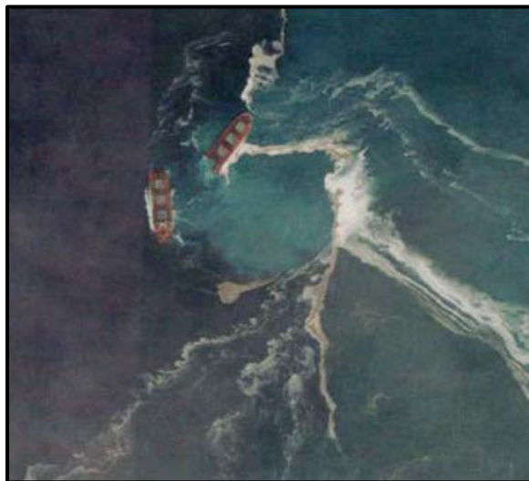
(12/13/04) The 738 foot freighter SELENDANG AYU ran aground near Skan Bay off Alaska's Unalaska Island. The ship snapped in two and spilled an estimated 41,000 gallons of oil into the ocean. This image of the wrecked freighter was captured by NASA's QuickBird satellite. (Photo: NASA)
