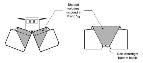
R.6(3)-3 Spaces open to the sea should not be excluded from the total volume of all enclosed spaces (V) if they are used for cargo and/or buoyancy purposes.
