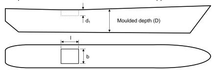
R.2(1)-4 In a ship having openings in the side of the ship below the uppermost deck, which are not closed but limited inboard by weathertight bulkheads and decks, the deck below such openings should be considered the upper deck.
