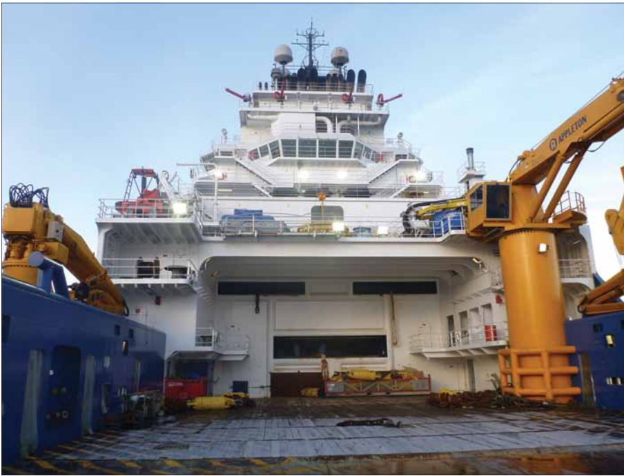
This photo looking forward toward the after superstructure of the M/V Aiviq shows some of the complex systems aboard the vessel, such as towing, firefighting, and lifting equipment. U.S. Coast Guard photo.
