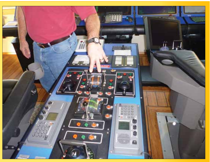
In the photo above, the bridge control equipment on the M/V Delta Mariner , and similar propulsion control equipment aboard the M/V Aiviq (right). Such complex, sophisticated equipment requires putting a comprehensive safety management system in place so the vessel's crew knows how to operate the systems under all kinds of expected conditions. U.S. Coast Guard photos.
