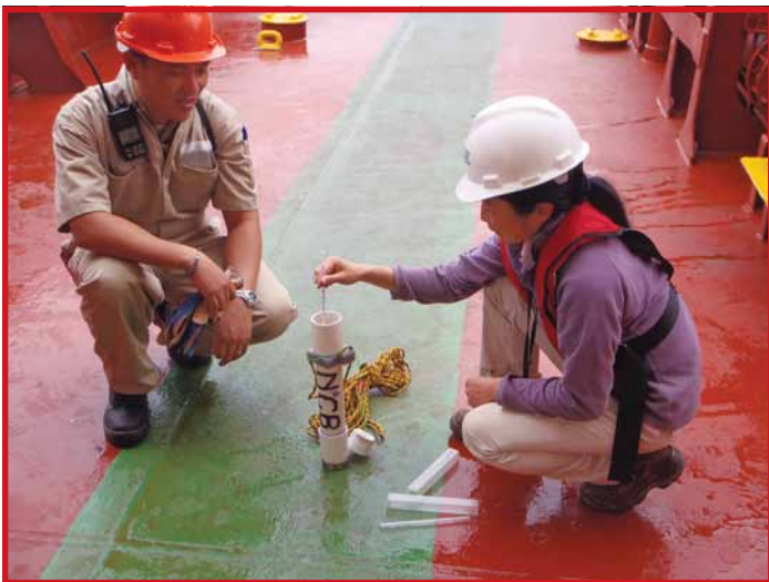
National Cargo Bureau surveyor Captain Emily Lai tests water density on a dry bulk ship. NCB surveyors work in the maritime domain on a daily basis. Photos courtesy of the National Cargo Bureau.
