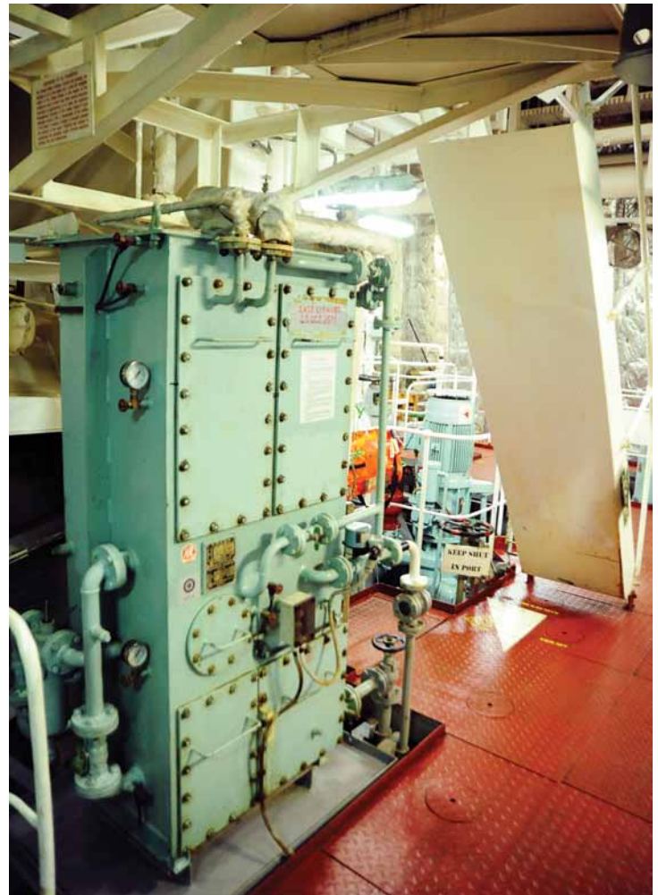
An oily water separator onboard a motor vessel in the Port of Los Angeles. (Not the vessel in question.) U.S. Coast Guard photo by Petty Officer Prentice Danner.
