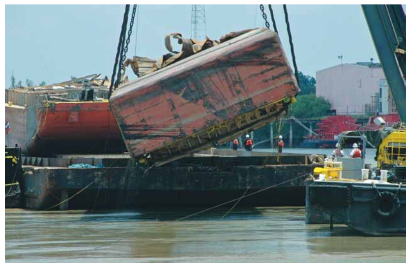
The fuel barge DM 932 is placed aboard the carrier barge as salvage operations of the wreck on the Mississippi River at New Orleans come to an end. The bow section of the barge was removed from the river Aug. 9, 2008. U.S. Coast Guard photo by Petty Officer Adam C. Baylor.
