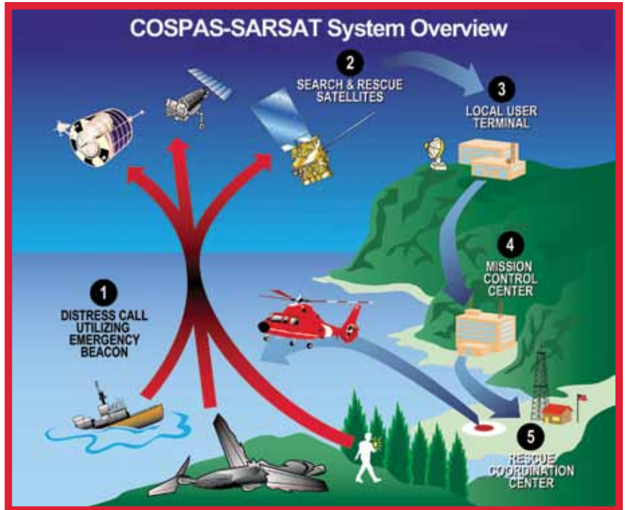
Cospas-Sarsat system overview. Diagram courtesy of U.S. SARSAT program.
