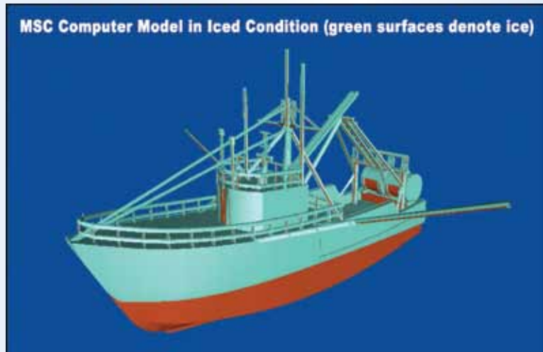
Marine Safety Center computer model in iced condition (green surfaces denote ice).
