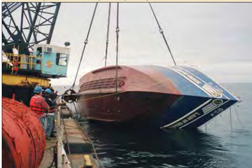
Vessel being loaded onto barge during salvage phase.
