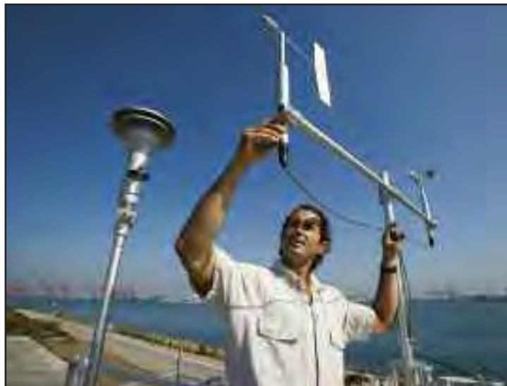
An air quality monitoring station at the Port of Long Beach is one of two such installations furnishing round-the-clock air pollution data posted on the port's Web site and that helps guide the port's air quality improvement efforts. Photo courtesy of Mr. Tim Rue, TRUE Photo, for the Port of Long Beach.
