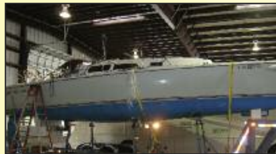
The same sailboat after the accident, with keel missing.
