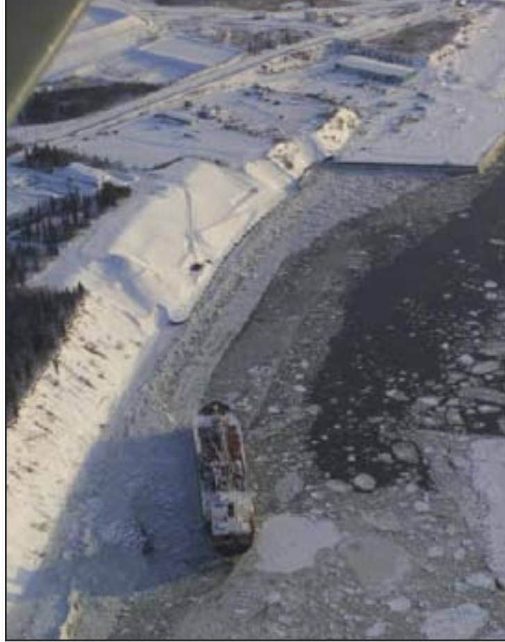
The vessel remained grounded for more than 24 hours. The outer hull of the vessel was pierced by the rocks, but the double hull acted as designed, preventing further spillage. USCG photo.
